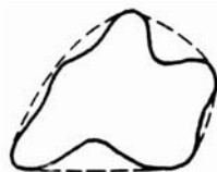
Figure 3.8 - Convex hull perimeter used during the mean Ferret diameter measurements [180].
