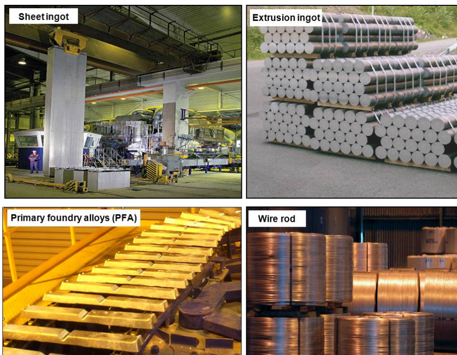
Figure 19 End products of primary aluminium casthouse [Kva11]
