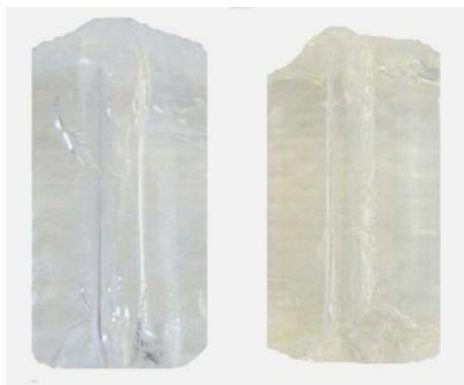
Figure 4.9 Photograph showing the appearance of hydrogels (M15DC05) obtained with 2 wt% of PI, irradiated 15.0 (left) and 20 min (right).
