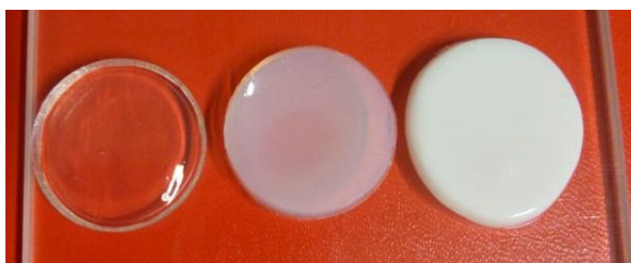
Figure 4.10 Photograph showing the conventional hydrogel (left; M15DC05) as well as the influence of crosslinker (middle; M15DC10) and porogen content (right; M15DC05PEG40) on the appearance of hydrogels.
