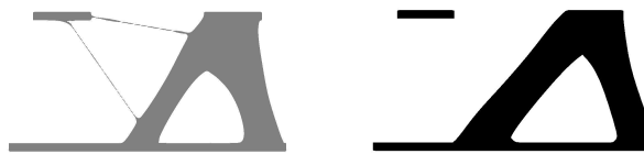
Figure 3.5: During the optimization process of the excess-probability model ( for \eta = 0.4 ), a focus on the right bearing manifests itself. This is due to the fact, that loadings on the right are smaller than the ones on the left, but occur with higher probability. This leads to decreasingly thin structures on the left, until those are completely neglected by performing a topological optimization step. The final result is shown on the right.
