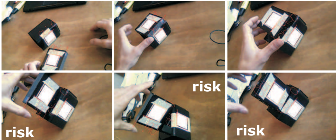
Figure 9.14: The stack-it-safely task: The labeled pictures show risk situations (upward stacking of the narrow object). The others show normal situations (stacking objects located somewhere else or in correct position at the top of the other object) (Ertle et al., 2012b).
