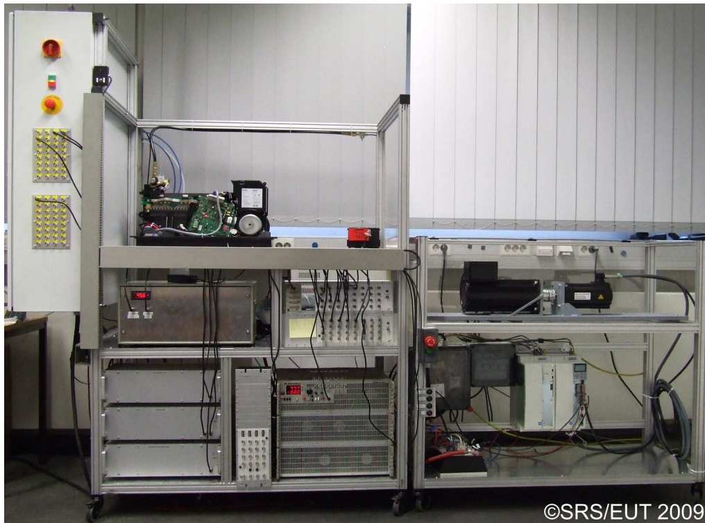
Figure 3.1: Fuel cell/supercapacitor-based Hardware-in-the-Loop (HiL) test rig ( [Özb10], [MOS09], [MOS10] )
