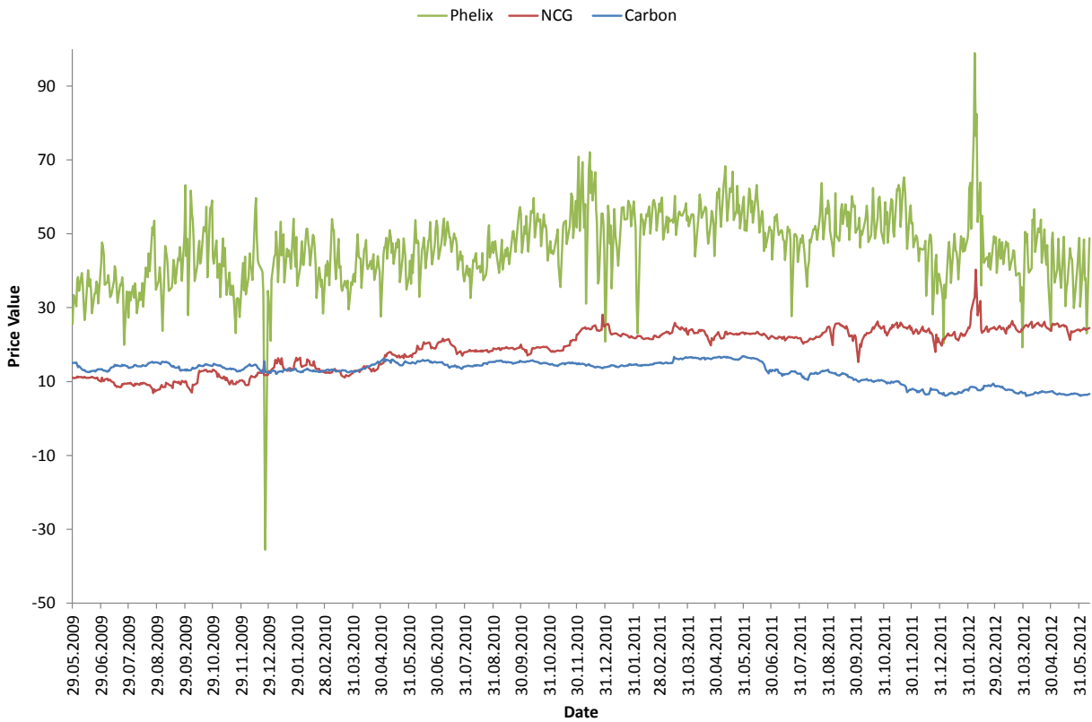
Figure 5.2: Evolution of the power (base load), gas, and carbon prices between 25.09.2009 and 08.06.2012.
