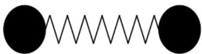
Figure 2.1: Balls and spring model. In MM methods the molecules are represented as systems of solid spheres connected via springs.
