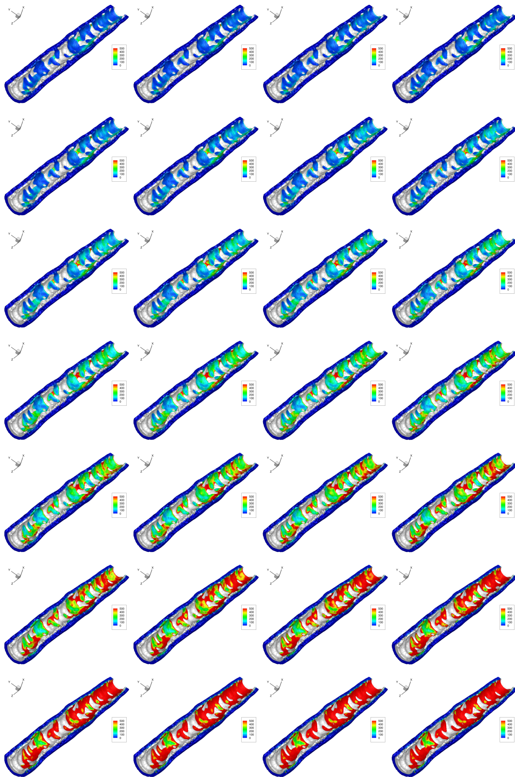
Figure 3.9: Model artery 2; 13 million d.o.f.; \Psi_A Set-2; Von Mises equivalent stresses on the internal surface of the media component; Loadsteps 40 to 67. This corresponds to an internal normal pressure increasing from 10 [mmHg] to 500 [mmHg].
