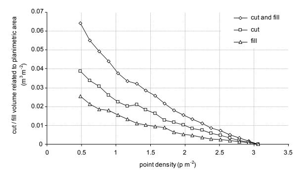
Figure 3.3: Terrain model surface error (per unit stream area) against survey point density.
