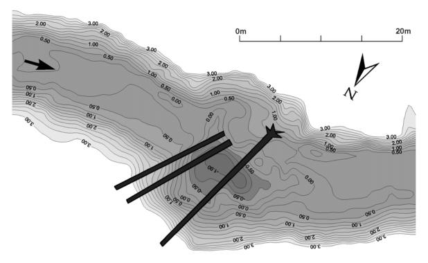
Figure 3.4: Contour map of Berkel1 LW section 3D-model. Height above / below mean stream bed height is given in meters. Stream bed area one standard deviation above / below mean depth of stream bed (0.5 m) is defined as bar and pool respectively. Pool is located downstream of the first large fallen tree, which is located on the stream bed. Sketch of the large fallen trees is not to scale; flow is from left to right.
