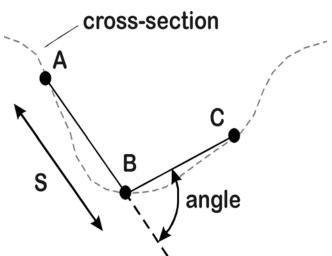
Figure 3.5: Measurement of cross-section angle for AMT-Analysis.
