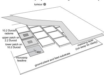
This contribution presents theoretical (using FDTD) and practical results (using a phantom) from a stacked-patch antenna array.
