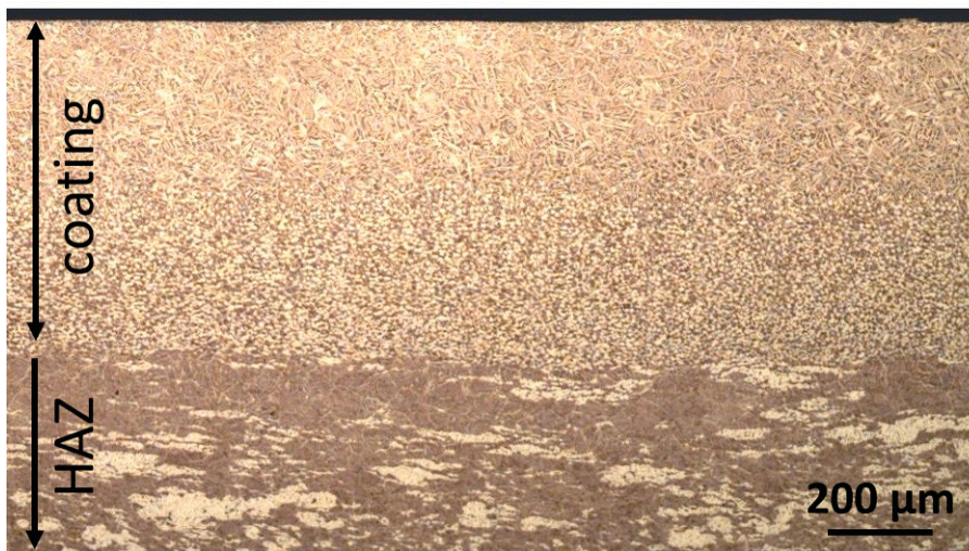
Figure 25: Detail from a cross section of a single layer NiAl-bronze FS coating showing also part of the heat affected zone (HAZ) in the substrate.
