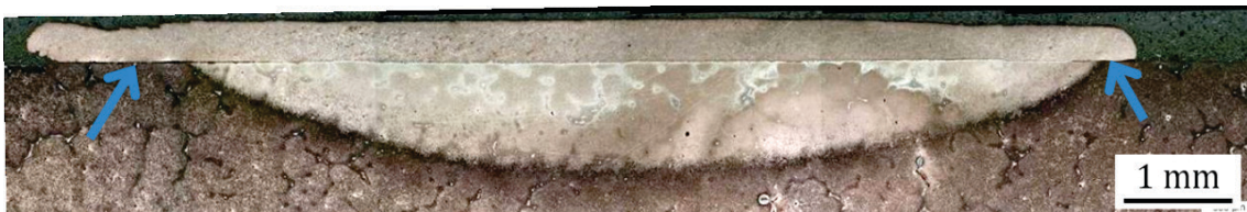
Figure 11: Cross section of a single layer CP4M coating, showing substrate, HAZ and coating with lack of fusion zones (arrows).
