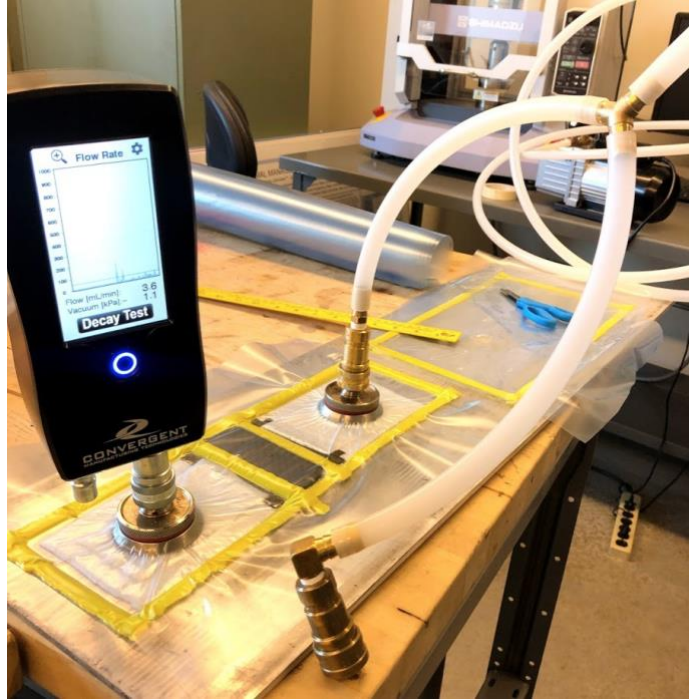
Figure 7. Cirrus apparatus with the COHO mass flow meter attached to the left side vacuum port.
