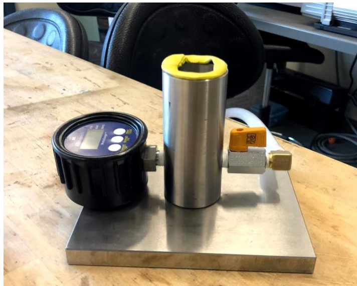
Figure 4. Sealant tape placed on the rim of the cylinder to allow for mounted sample to attach to the apparatus.
