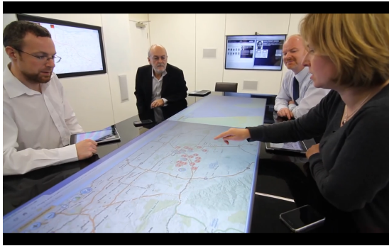
Figure 5: The 108 inch multi-touch table at Edinburgh Napier University, part of their Interactive Collaborative Environment (ICE). Images courtesy of Institute for Informatics and Digital Innovation.
