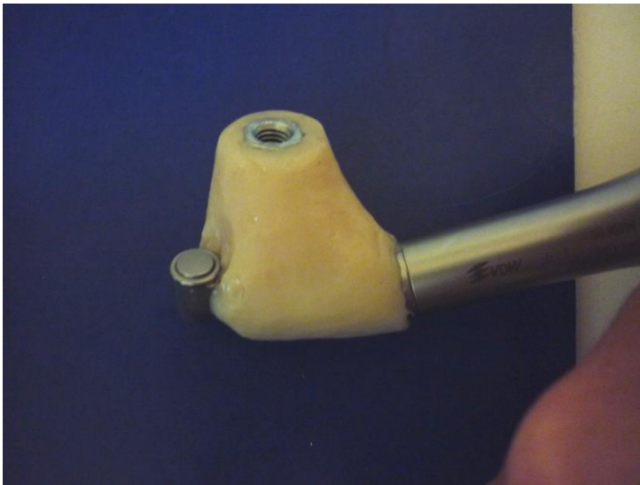
Fig 27. The acrylic jig secure on the handpiece. The nut in the jig accommodates the vertical stop screw (photographed by the author).
