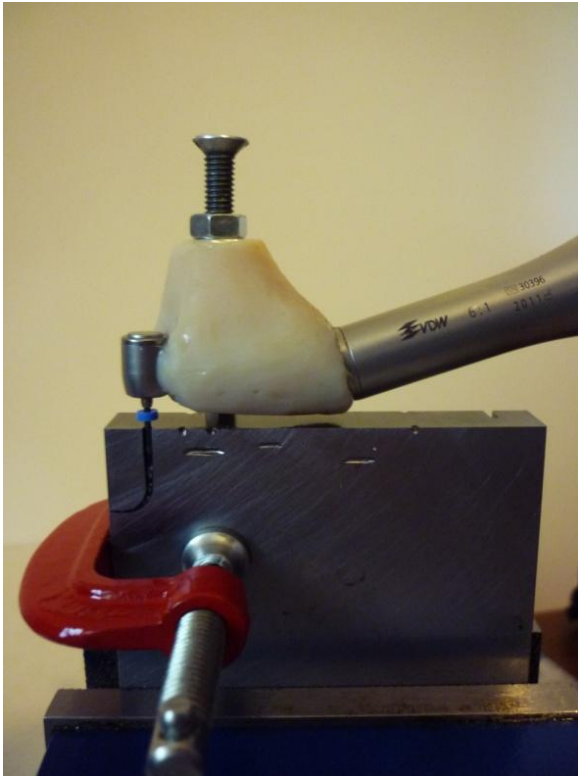
Figure 28. The full test assembly with vertical stop screw and locking nut (photographed by the author).
