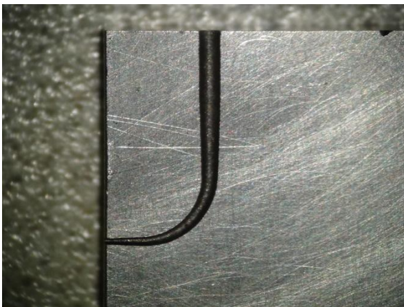
Figure 25. The artificial canal in the steel block (photographed by the author).
