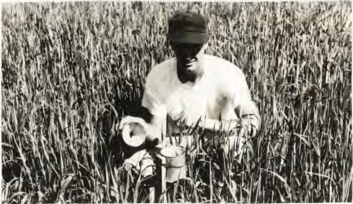
Figure 7. Cans used for catching water to measure application. A funnel was soldered flush with the top of each can to decrease evaporation losses. Also, note that the top of the can is kept on the same level as the crop height.
