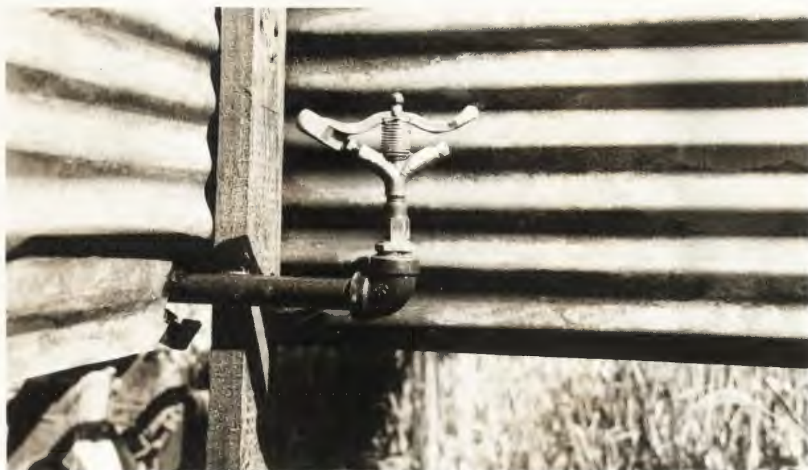
Figure 4. "Rain Bird" full-circle sprinkler used for applying water to plots, with shields in the background.
