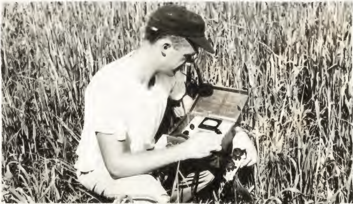
Figure 8. Coleman resistance bridge and switch used for reading the gypsum blocks. The bridge was calibrated to read blocks directly in atmospheres of tension.
