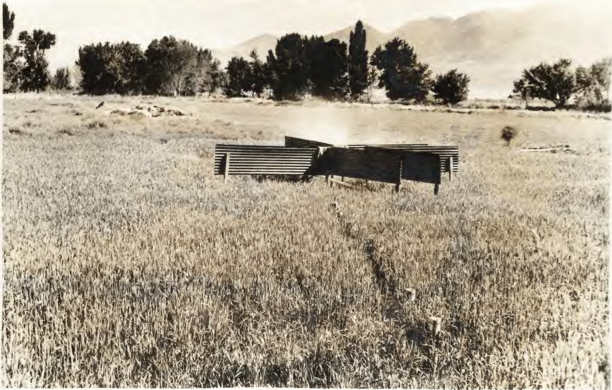
Figure 1. View of experimental area showing crop, shields and a row of cans on plot 1. Sprinkler is operating on plot 3 in the background.
