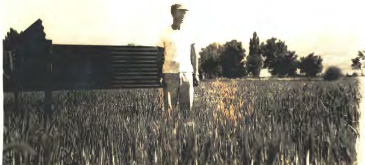
Figure 10. Growth of crop was "stunted" close to the shields on plot 2 because of an excess application of water, resulting in a large amount of deep percolation. This decreased crop growth and density did not extend to region where gypsum blocks were buried.
