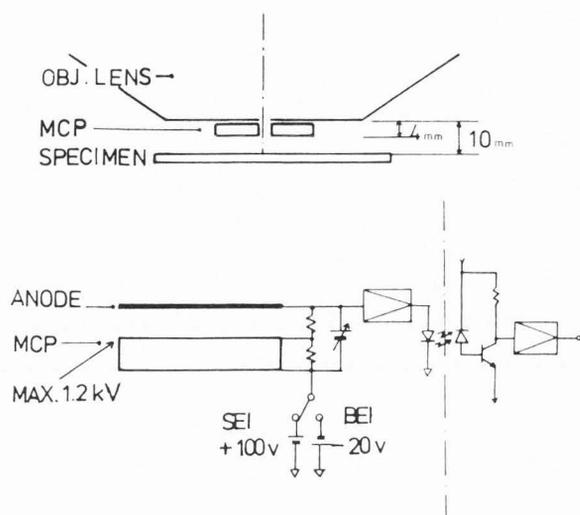
Figure 3. Microchannel plate detector geometry and electrical configuration.
