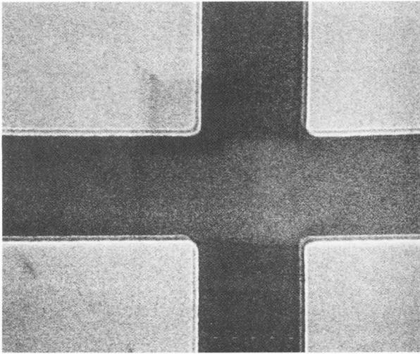
Figure 6. Micrograph of cross pattern (2 micron linewidth) obtained using MCP detector; 1 keV and 1 pA beam conditions.
