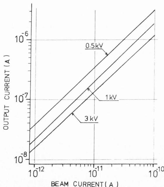
Figure 5. MCP detector output current versus primary beam current for 0.5, 1.0 and 3.0 keV beam voltage. Extraction voltage is 100V.
