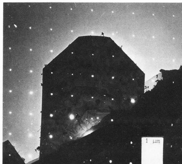
Fig. 14. Electron micrograph of molybdenum crystal with selected area diffraction pattern in the correct orientation by the use of rotation-free single-polepiece diffraction lens system.
