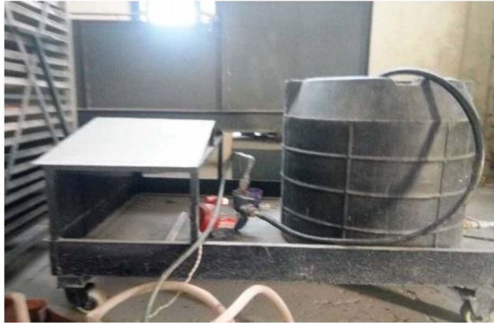
Fig. 3. Trolley arrangement with centrifugal pump and storage tank.
