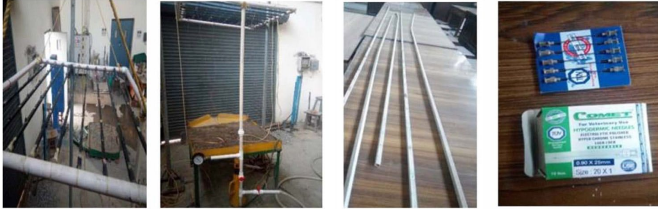
Fig. 2. Simulation system with lateral aluminum pipes and hypodermic needles.
