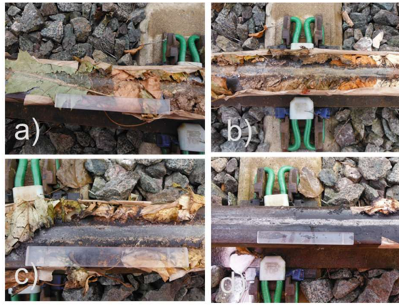
Figure 3 (a-d) Leaf layer generation after (a) 0 passes, (b) 2 passes (c) 5 passes and (d) post-test appearance
