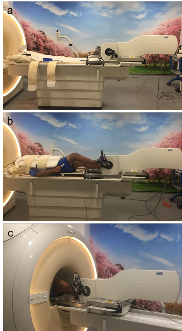
Fig. 1 The Lode BV supine cycle ergometer before (a), during set up (b) and during use (c)
