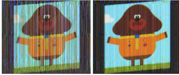
Fig. 7. (Left) Reconstructed image using the 256 \times 256 pixels scrambled Hadamard pattern with 1D uniformity correction. (Right) Same reconstructed image using 2D uniformity and contrast correction.
