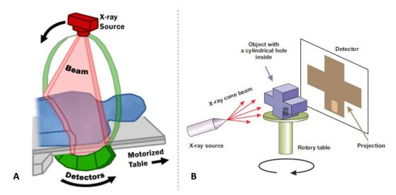
**Figure 3:** A: Setup of a medical CT scanner with a ring-shaped source-detector unit, from www.fda.gov; B: Setup of a typical lab-based micro-CT system. The X-ray source on the left and the detector on the right are stationary and the object in the centre is placed on a rotating stage, from Warnett et al. 2016.
