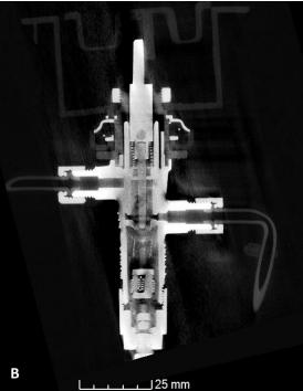
**Figure 43:** A: volume rendering and B: 2D vertical section through the gas valve scanned as part of the investigation of OP Bullfinch. The section shows the internal mechanism in a non-destructive way.
