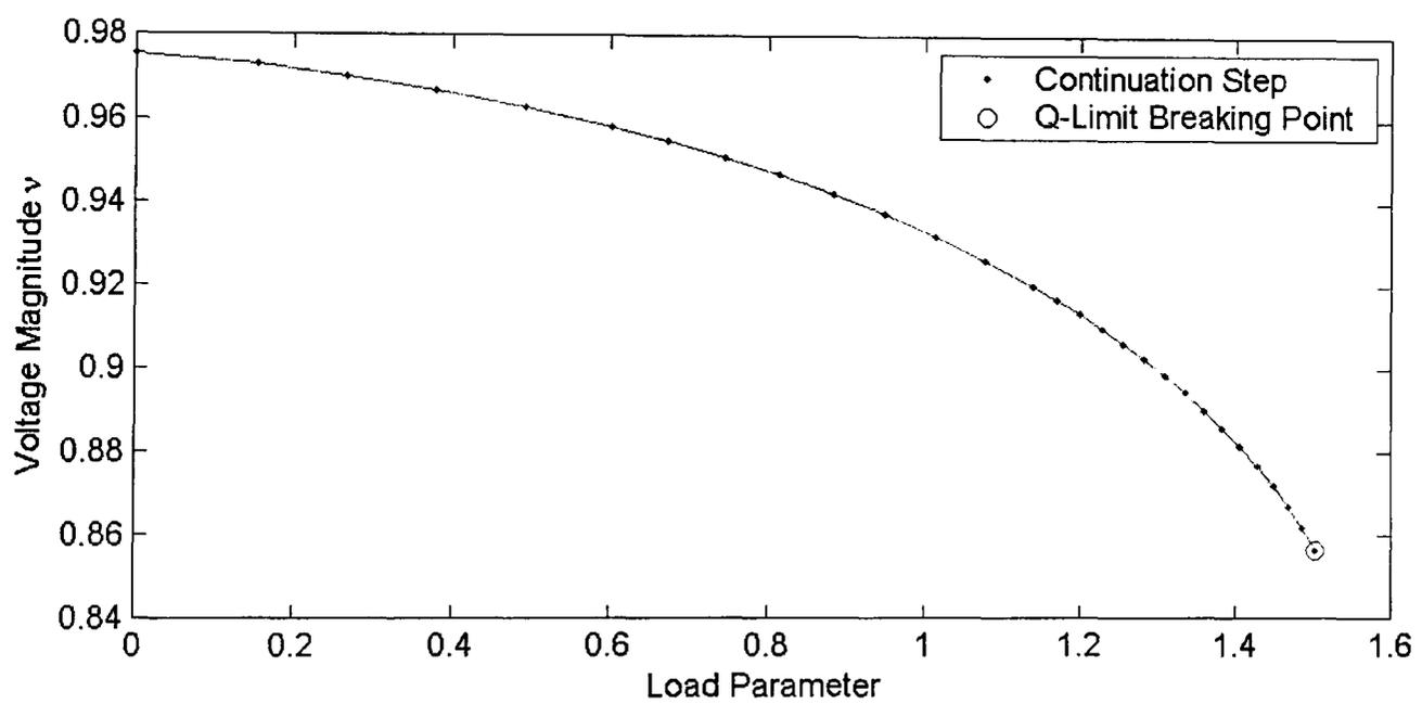
**Figure 6-3-b: Varying multiple load buses of IEEE 9 bus system using ECPF**
