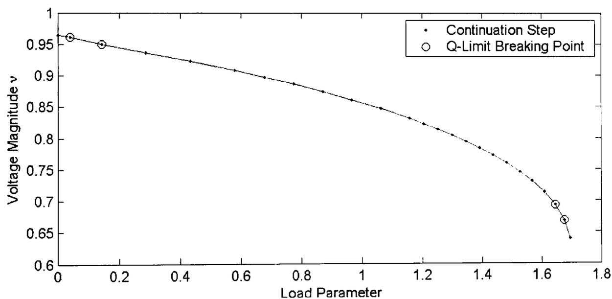
**Figure 6-9-b: Varying single load bus of NGC 61 bus system using ECPF**
