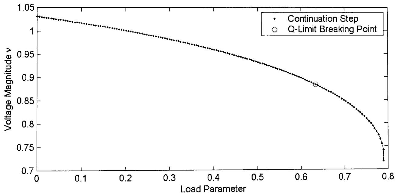
**Figure 6-11-a: Varying multiple load buses in area one of NG 953 using CCPF**
