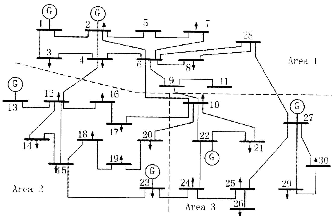
**Figure 6-4: Illustration of IEEE 30 Bus System**
