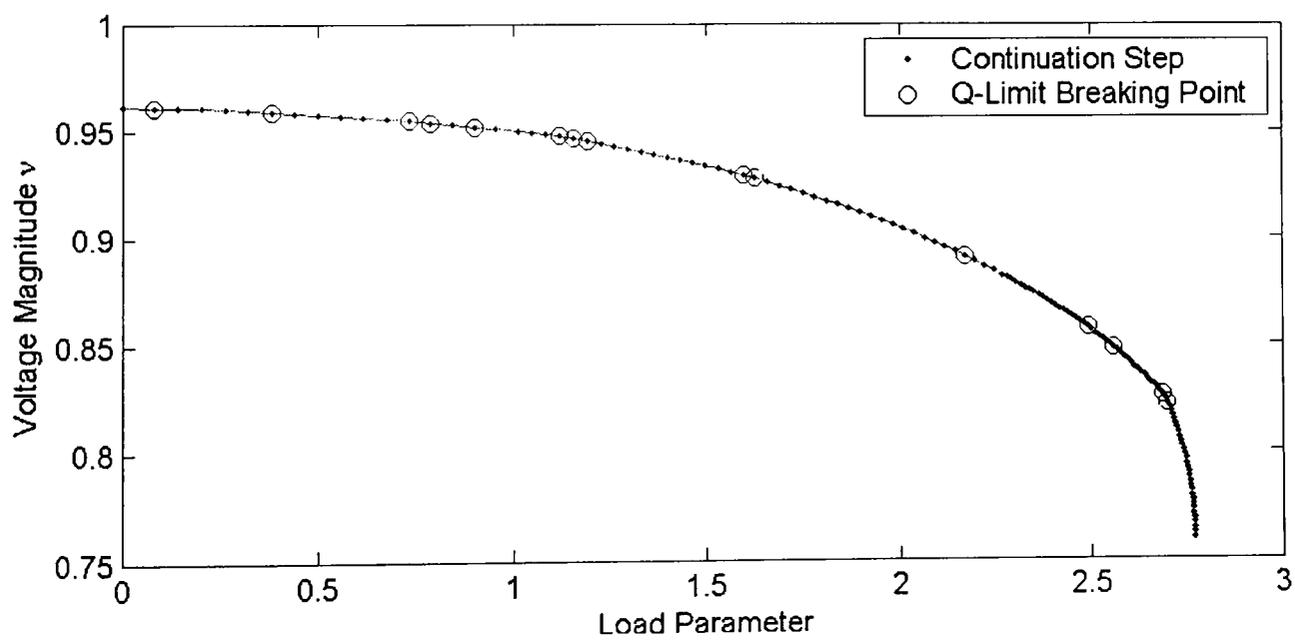
**Figure 6-8-b: Varying multiple load buses of IEEE 118 bus system using ECPF**
