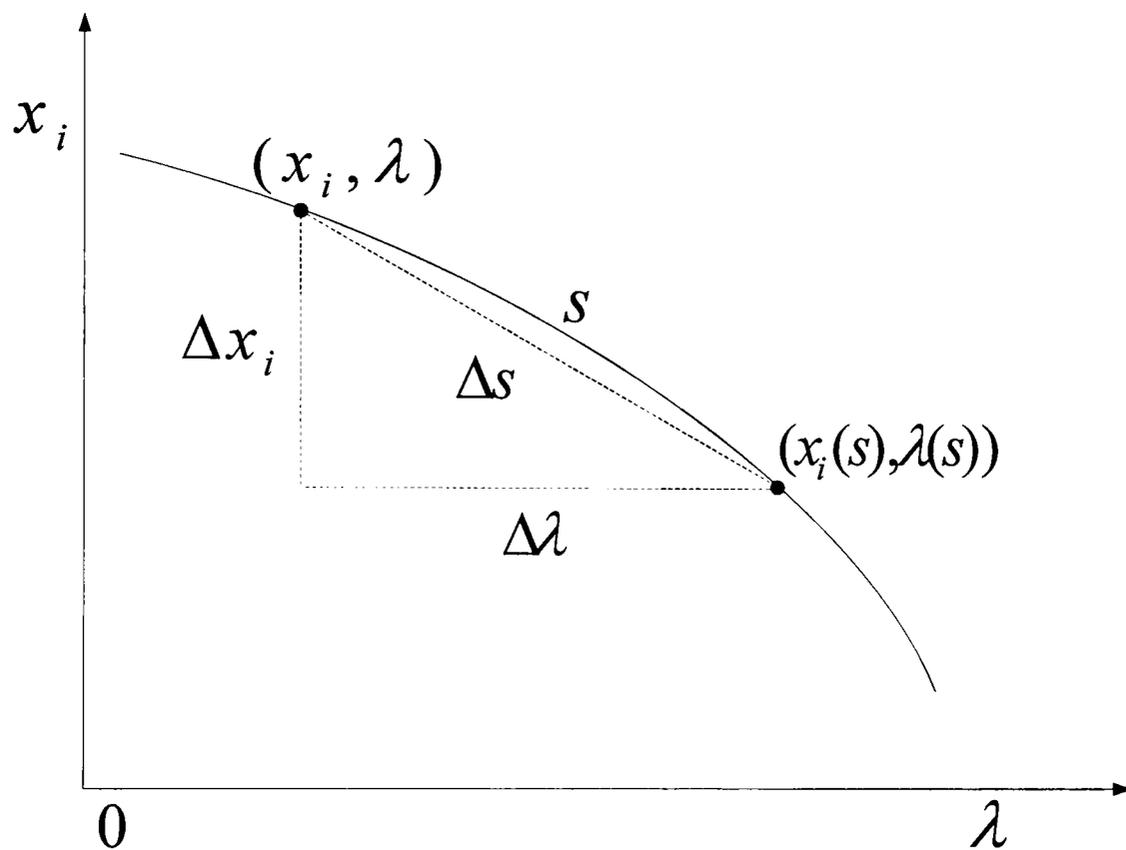
**Figure 2-1: Geometrical Representation of CPF Variables**
