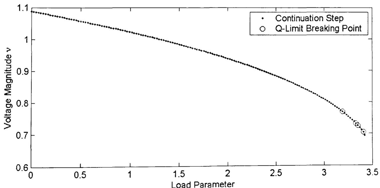
**Figure 6-13-a: Varying multiple load buses in area two of NG 953 using CCPF**
