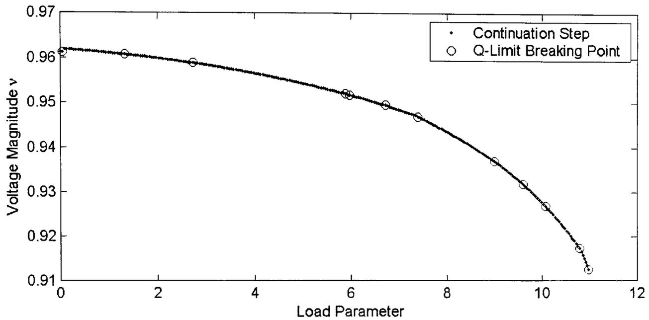
**Figure 6-7-a: Varying single load bus of IEEE 118 bus system using CCPF**
