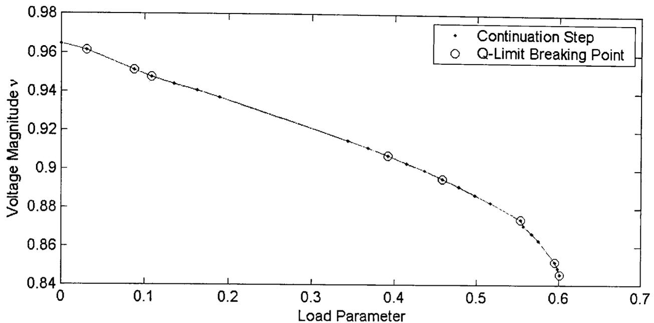
**Figure 6-10-c: Varying multiple load buses of NGC 61 bus system using GCPF**
