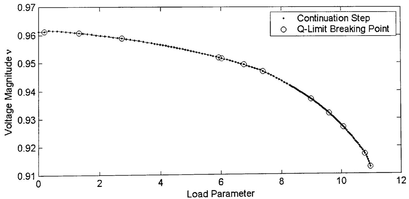
**Figure 6-7-b: Varying single load bus of IEEE 118 bus system using ECPF**
