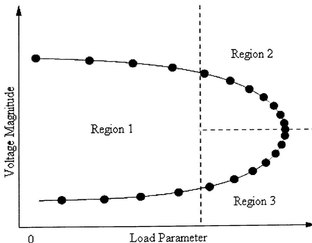
Figure 3-2: Decomposition of PV curve for Step-size Control
