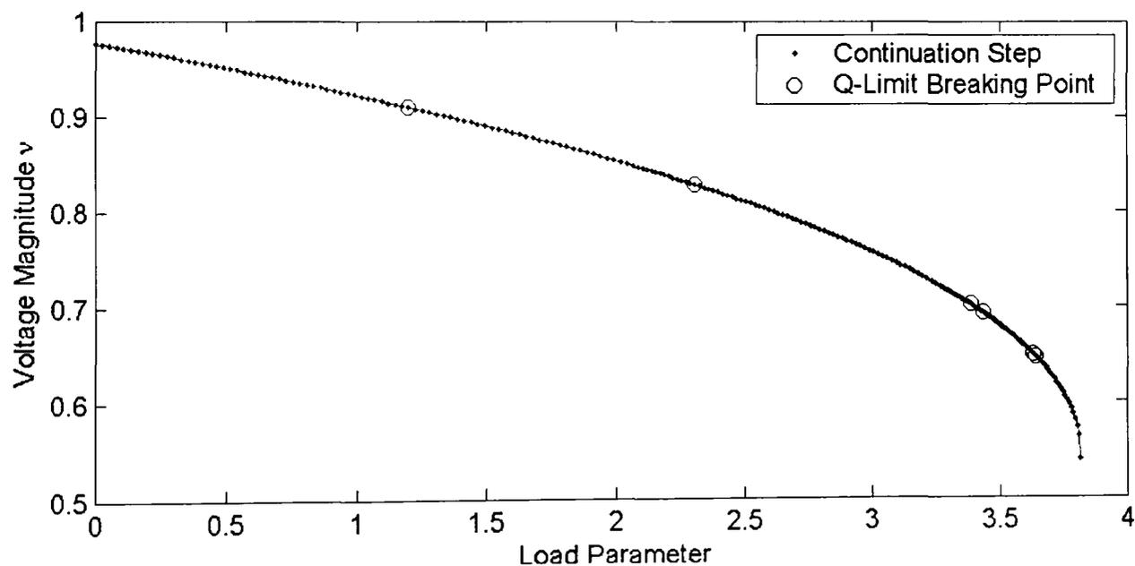
**Figure 6-14-b: Varying multiple load buses in area three of NG 953 using E CPF**
