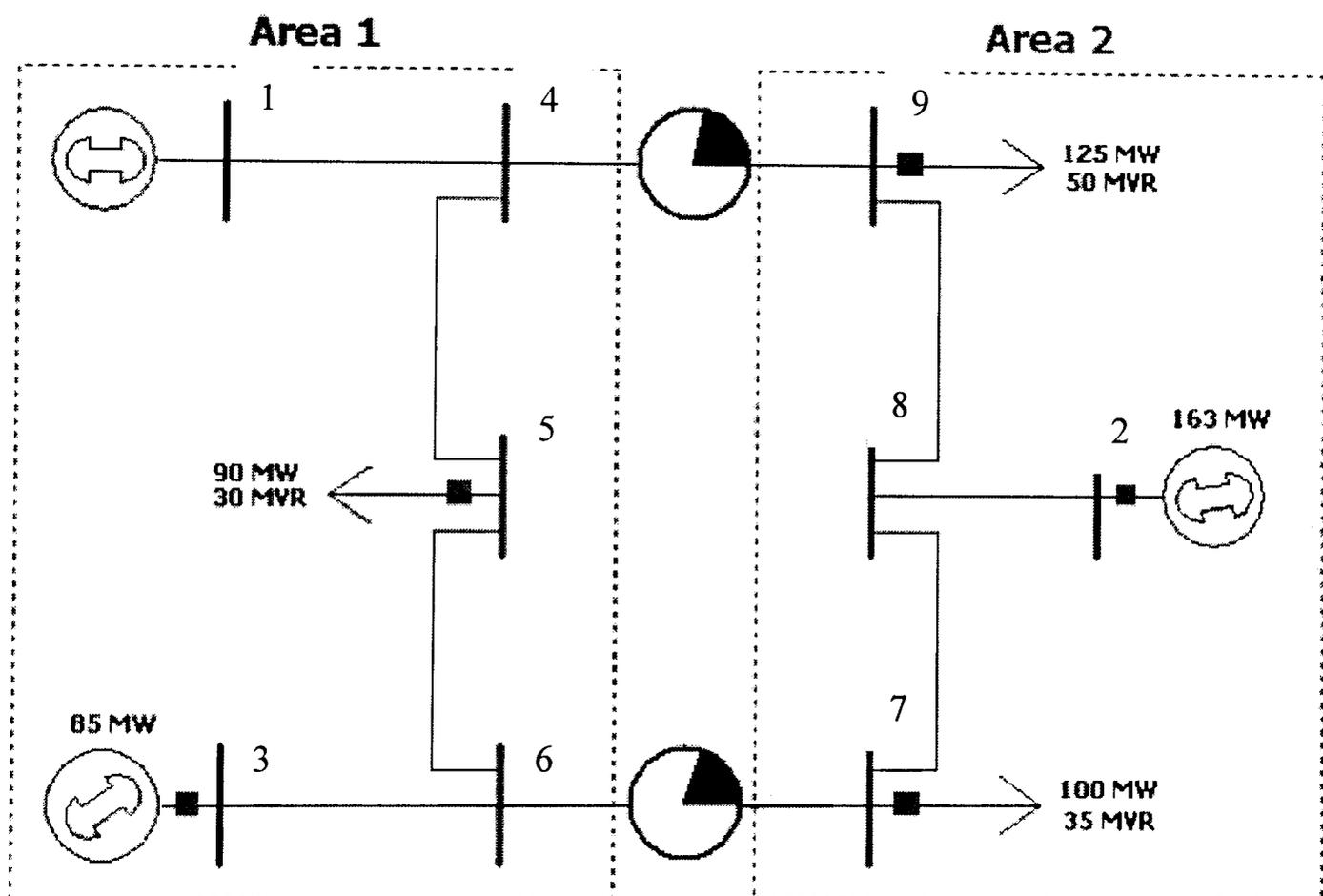
Figure 6-1: Illustration of IEEE 9-bus system
