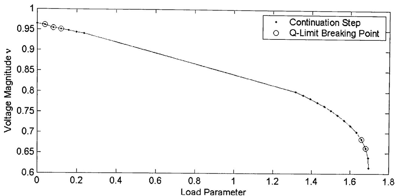
**Figure 6-9-c: Varying single load bus of NGC 61 bus system using GCPF**
