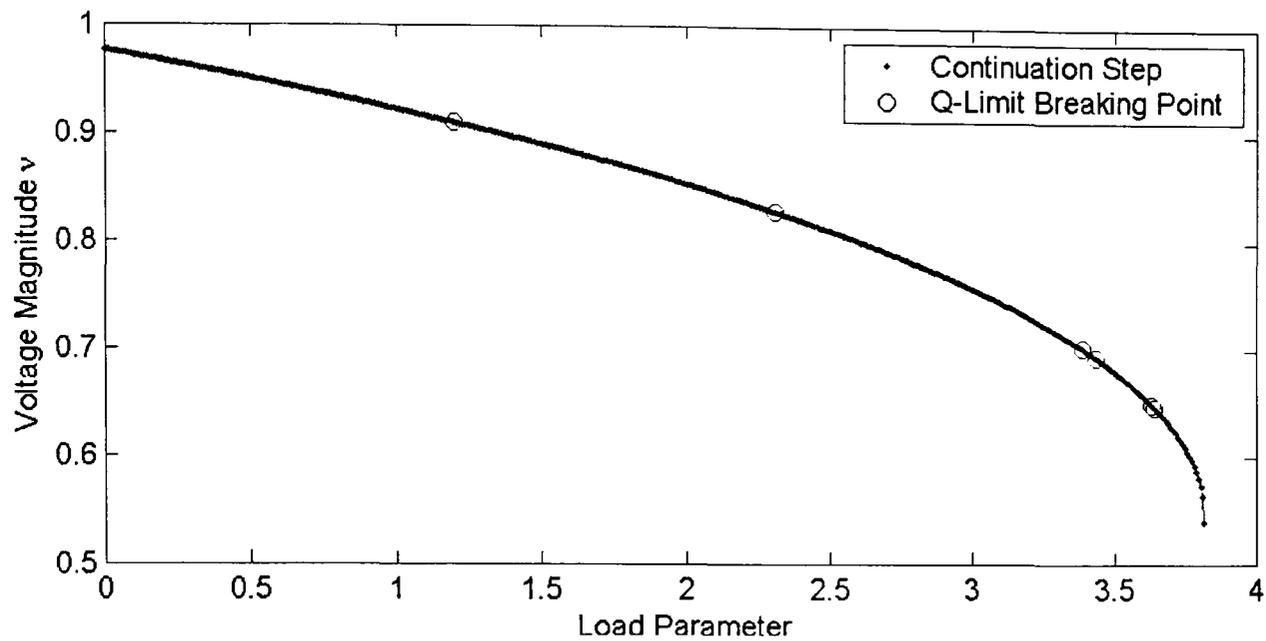
**Figure 6-14-a: Varying multiple load buses in area three of NG 953 using CC PF**
