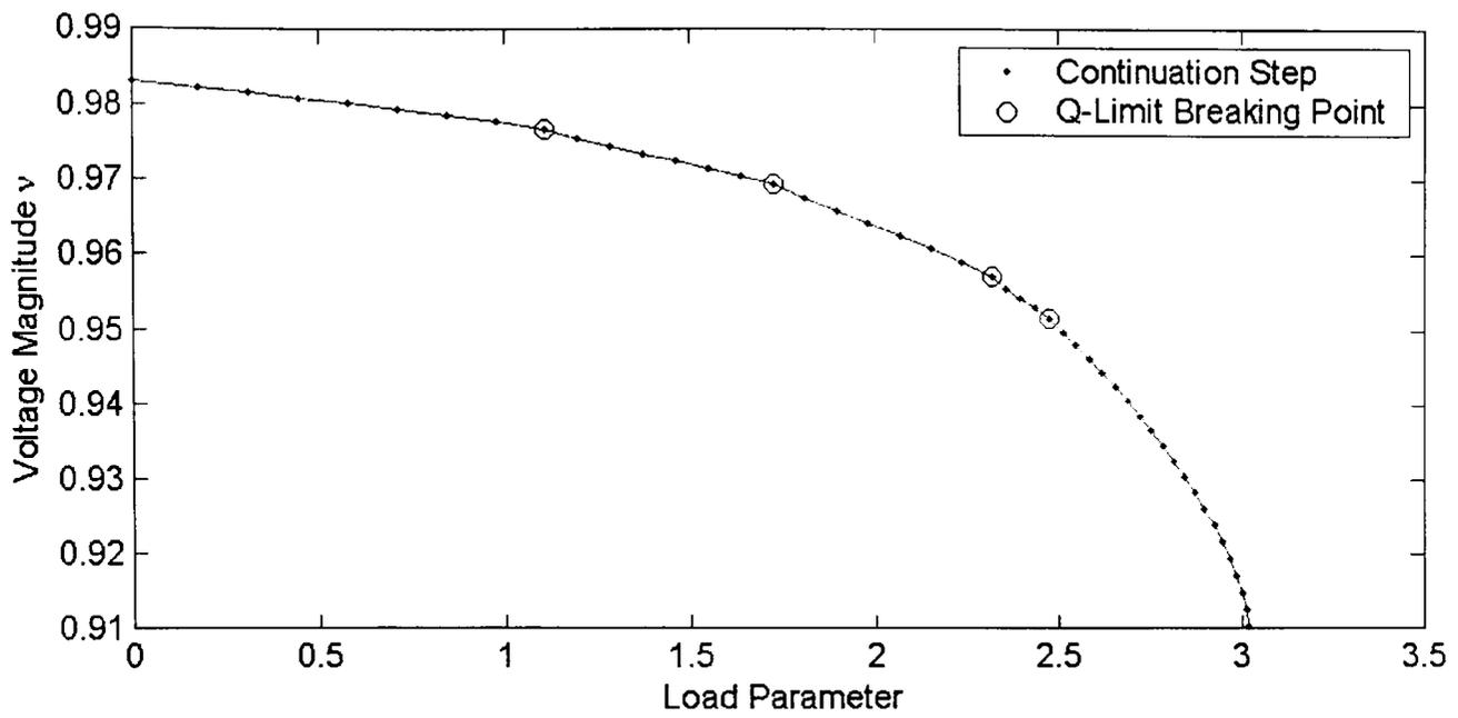
**Figure 6-6-b: Varying multiple load buses of IEEE 30 bus system using ECPF**
