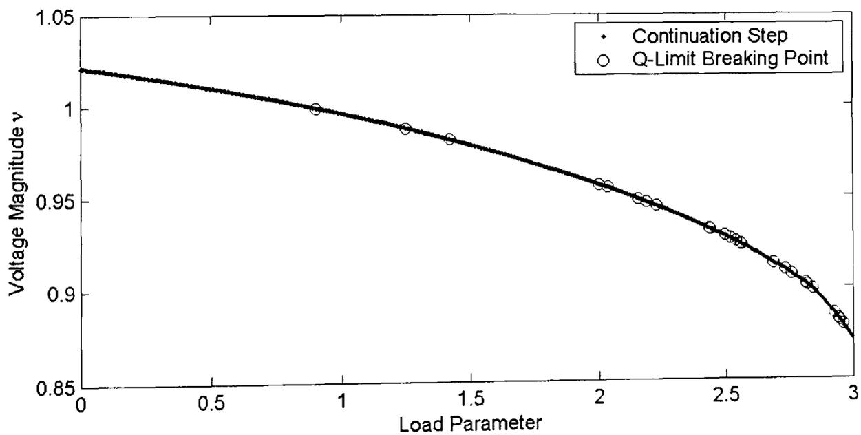
**Figure 6-17-a: Varying multiple load buses in area five of NG 953 using CCPF**
