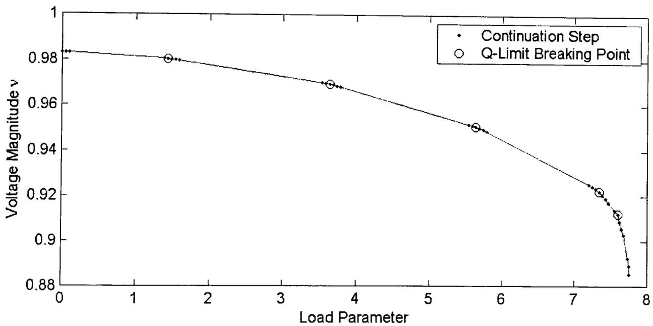
**Figure 6-5-c: Varying single load bus of IEEE 30 bus system using GCPF**
