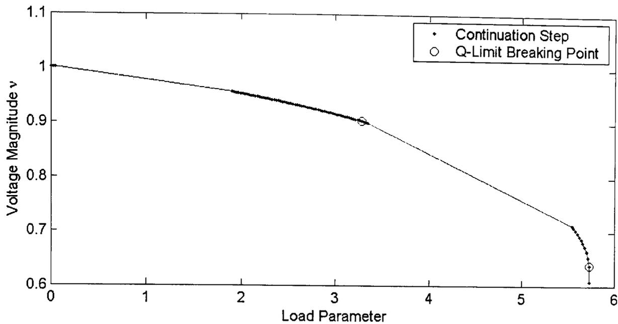
**Figure 6-16-c: Varying multiple load buses in area four of NG 953 using GCPF**
