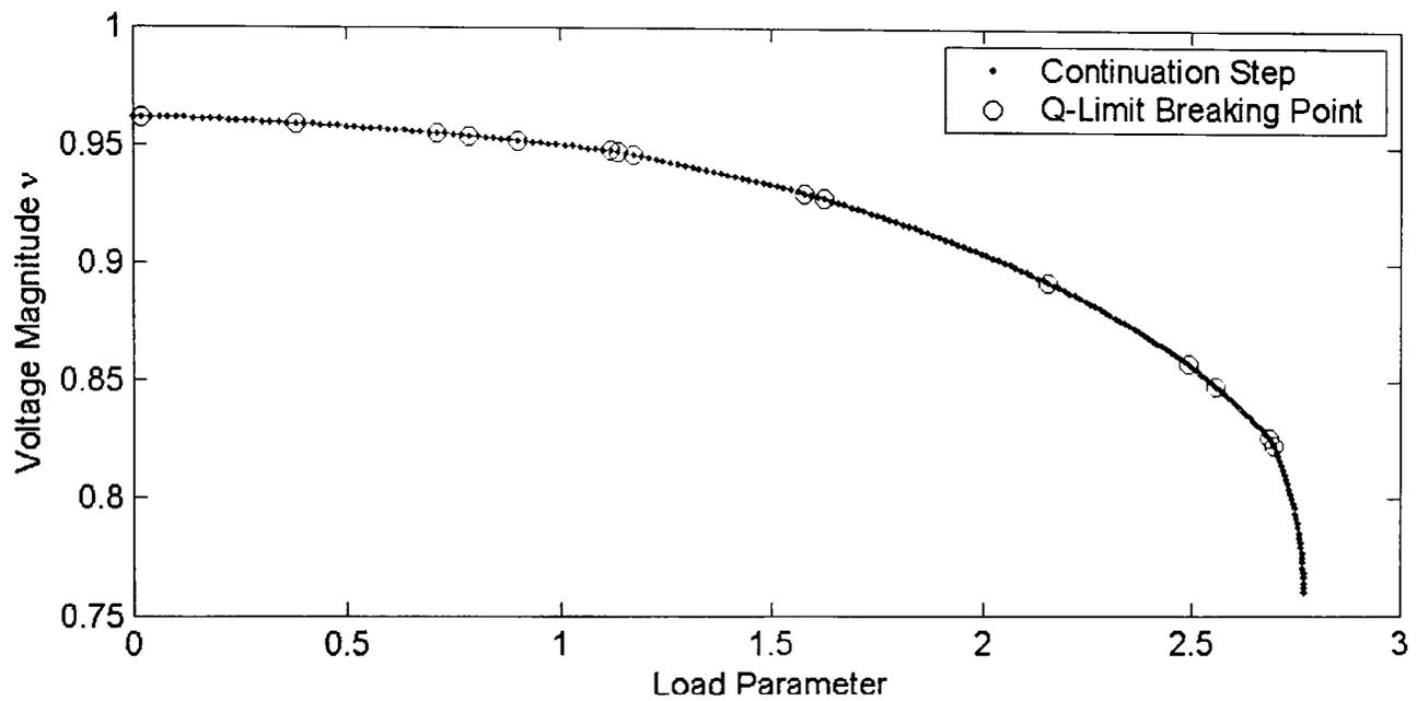
**Figure 6-8-a: Varying multiple load buses of IEEE 118 bus system using CCPF**
