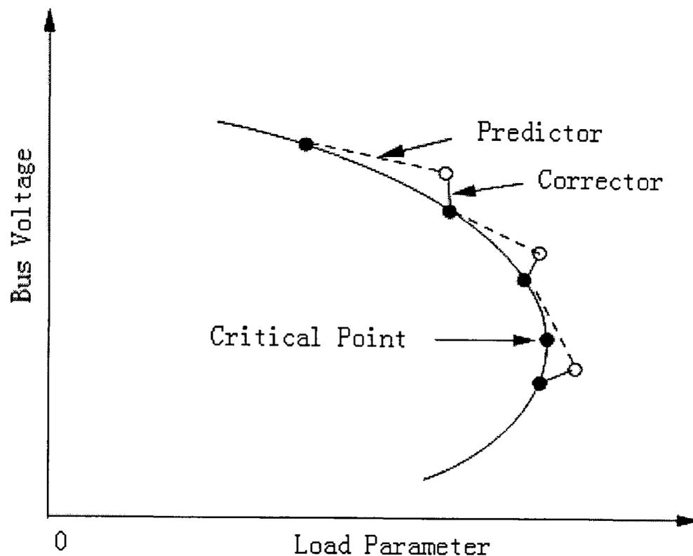
**Figure 2-3: An illustration of the predictor-corrector scheme used in CPF**
