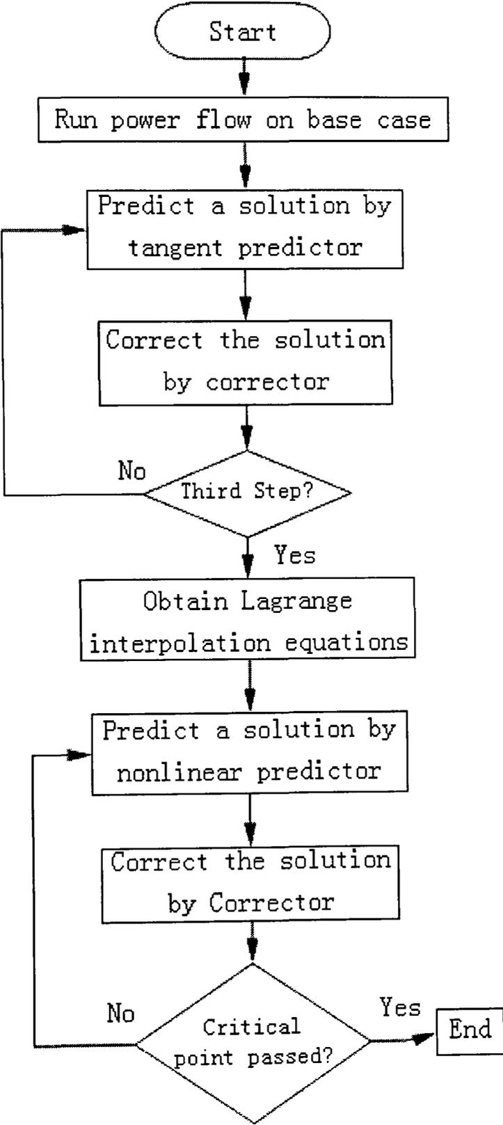
**Figure 3-1: Flowchart of CPF with nonlinear predictor**
