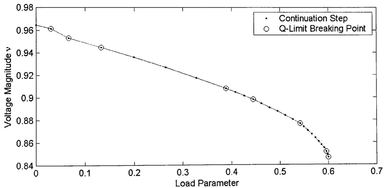
**Figure 6-10-b: Varying multiple load buses of NGC 61 bus system using ECPF**
