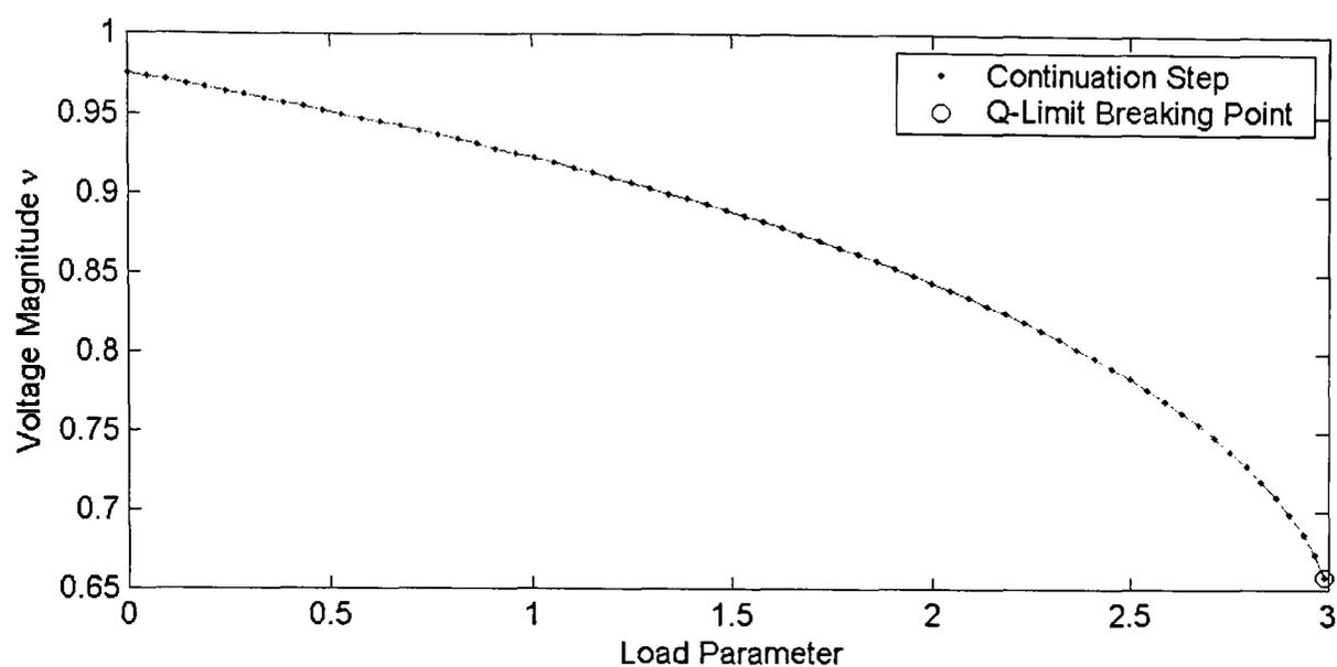
**Figure 6-2-a: Varying single load bus of IEEE 9 bus system using CCPF**
