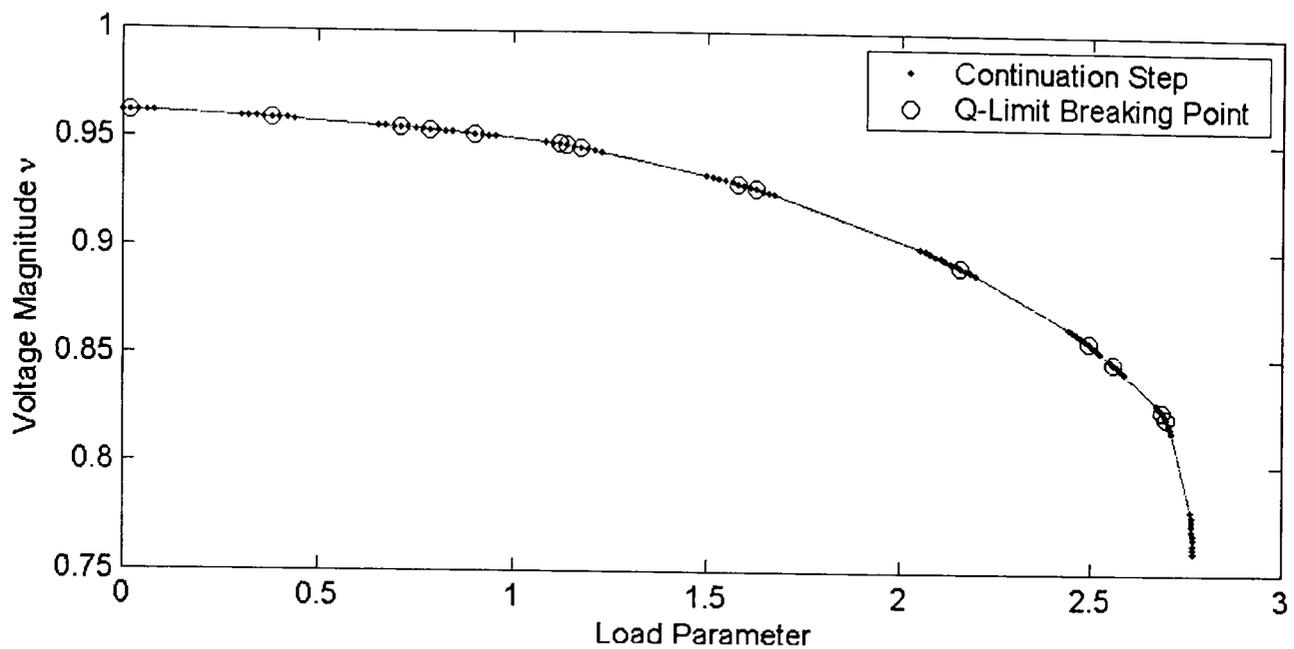
**Figure 6-8-c: Varying multiple load buses of IEEE 118 bus system using GCPF**
