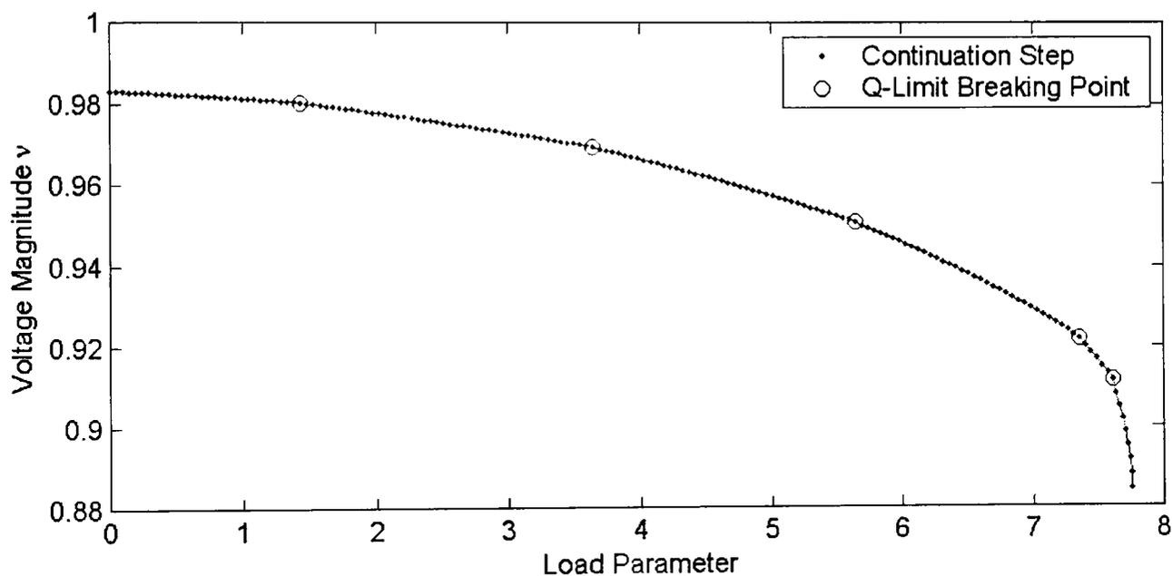
**Figure 6-5-a: Varying single load bus of IEEE 30 bus system using CCPF**
