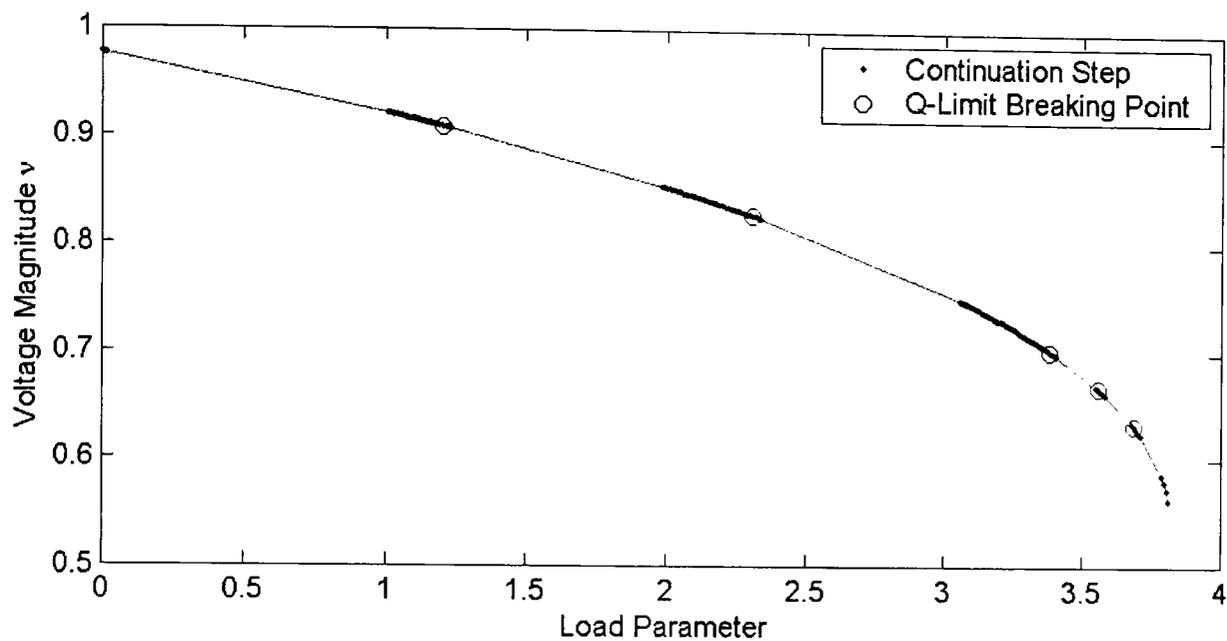
**Figure 6-14-c: Varying multiple load buses in area three of NG 953 using GCPF**
