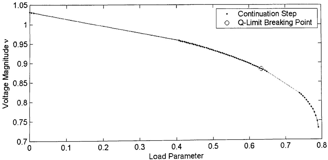
**Figure 6-11-c: Varying multiple load buses in area one of NG 953 using GCPF**
