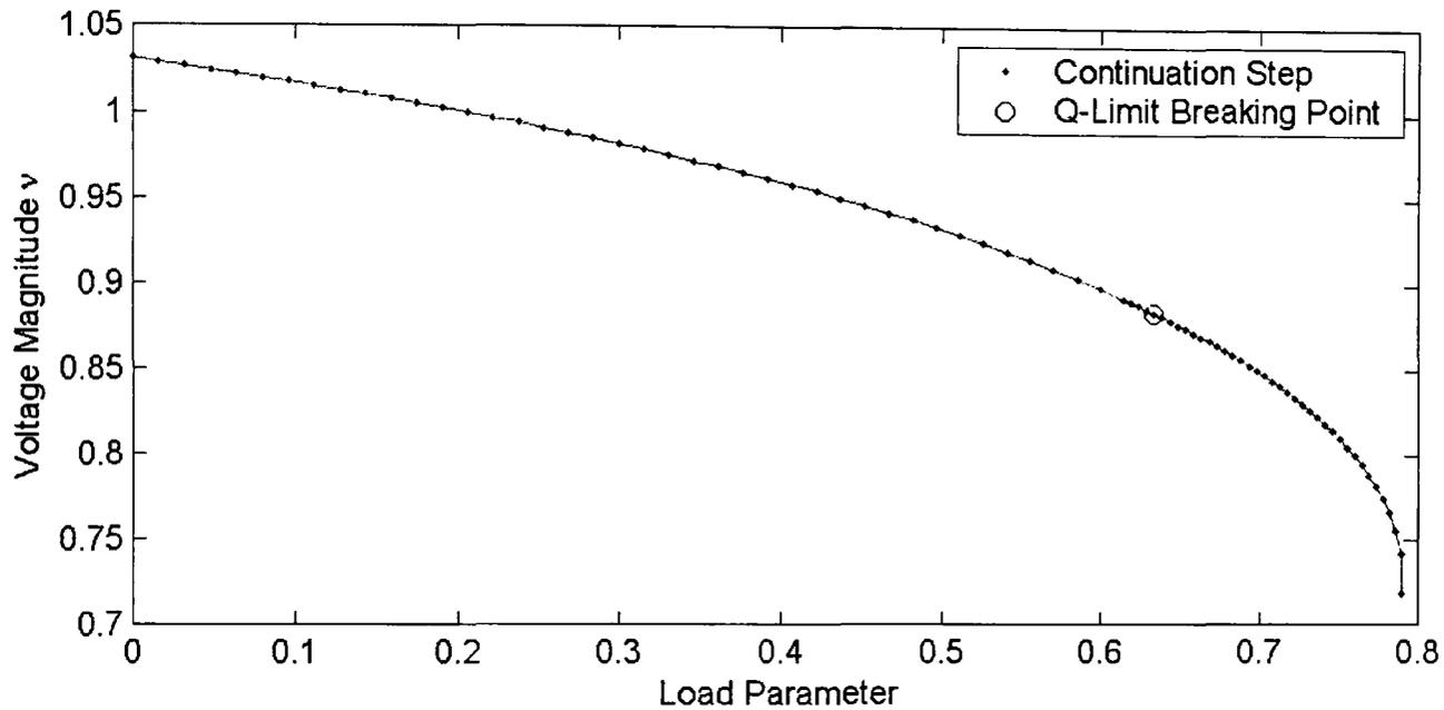
**Figure 6-11-b: Varying multiple load buses in area one of NG 953 using ECPF**
