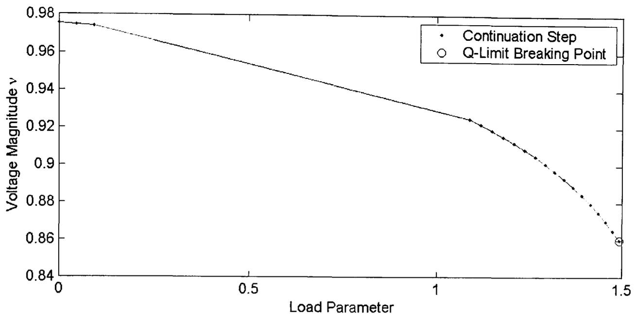
**Figure 6-3-c: Varying multiple load buses of IEEE 9 bus system using GCPF**
