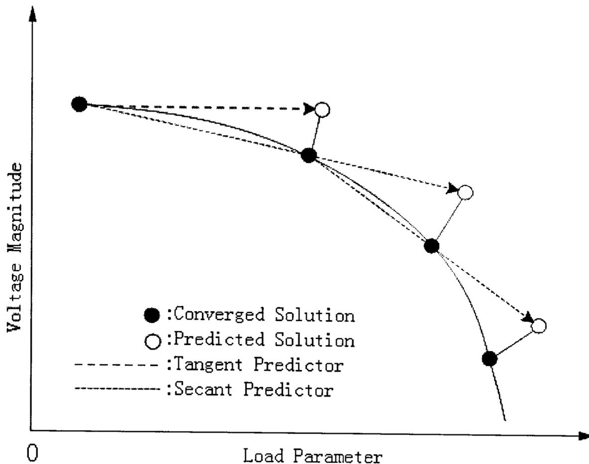
**Figure 2-2: Tangent and Secant Methods**
