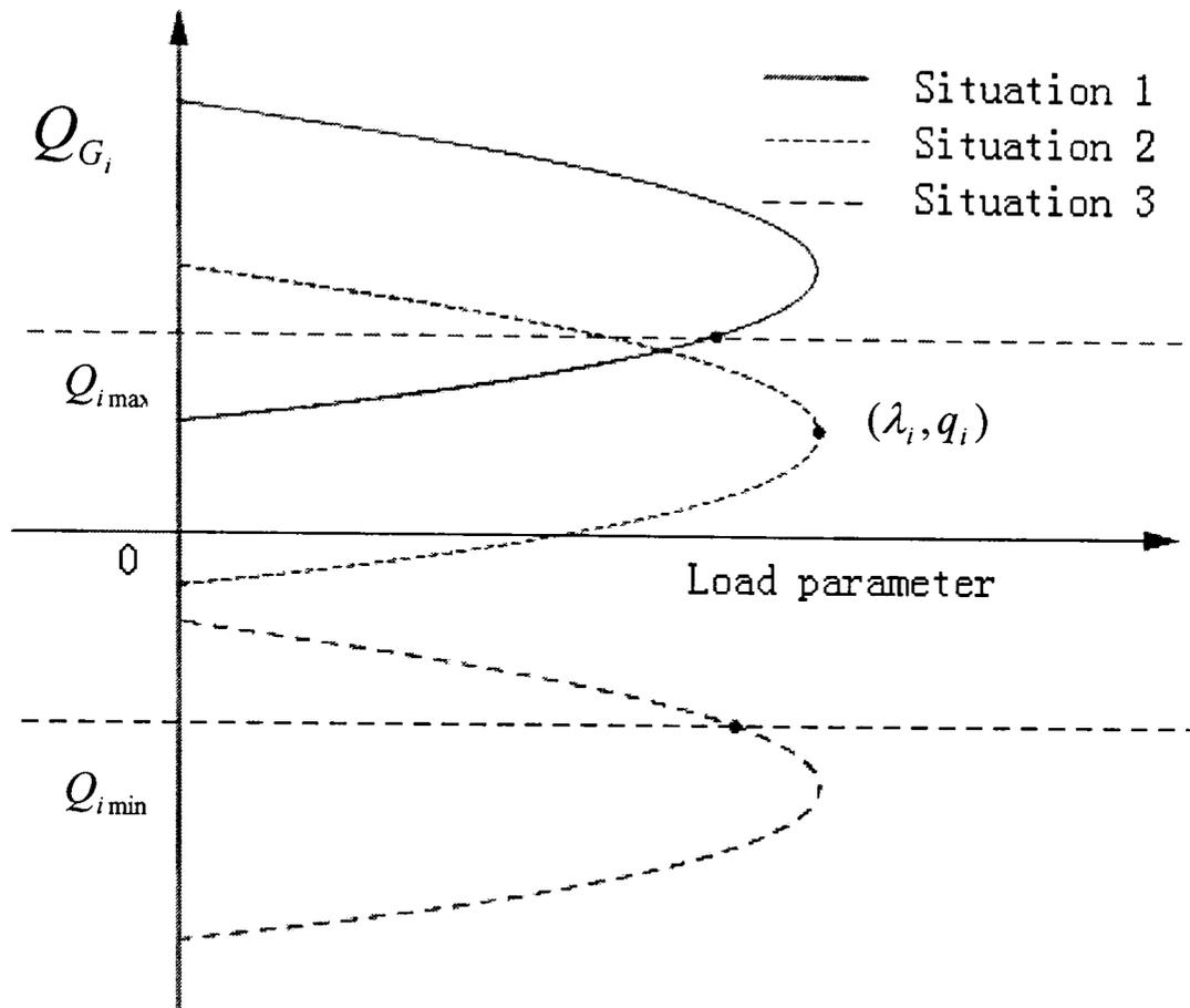
**Figure 3-3: Extreme value points and Q-Limit Situations**
