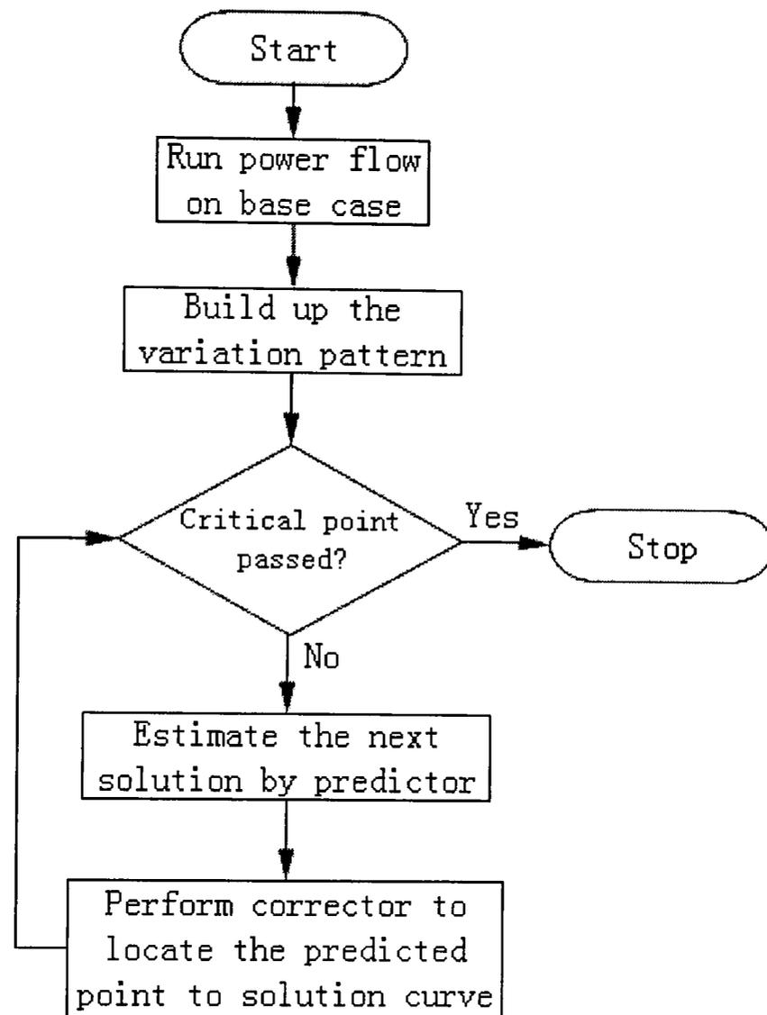
**Figure 2-4: Illustration of algorithm of predictor-corrector scheme of CPF**
