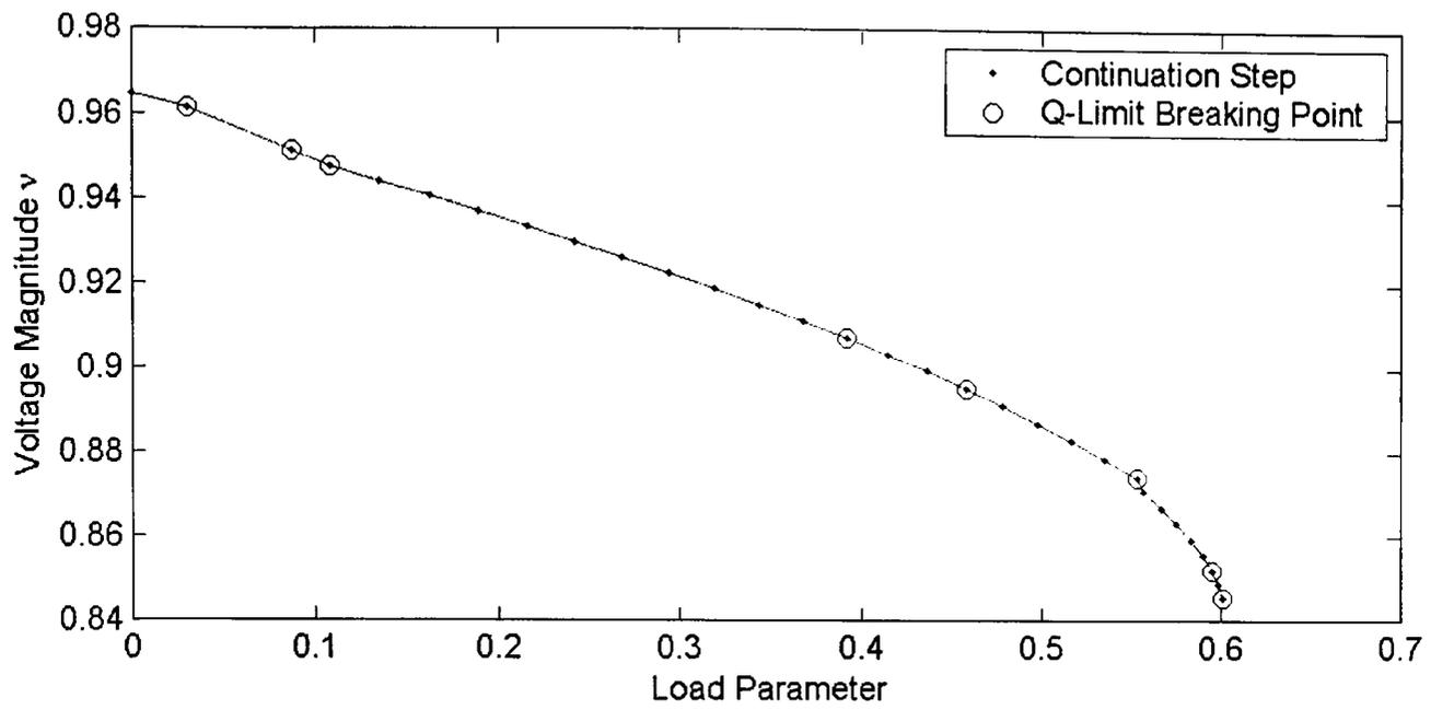
**Figure 6-10-a: Varying multiple load buses of NGC 61 bus system using CCPF**
