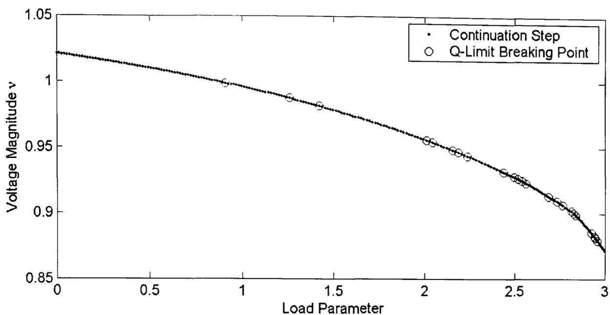
**Figure 6-17-b: Varying multiple load buses in area five of NG 953 using ECPF**
