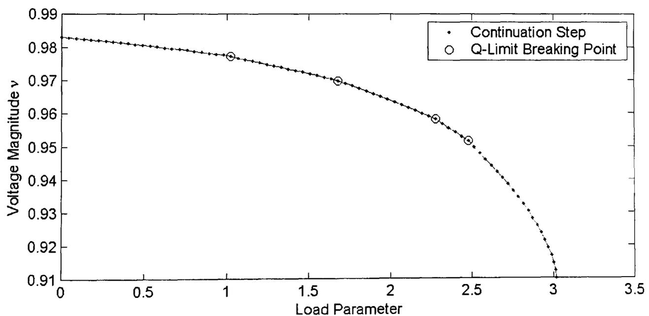
**Figure 6-6-a: Varying multiple load buses of IEEE 30 bus system using CCPF**
