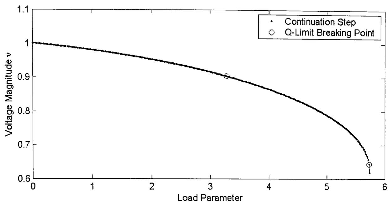
**Figure 6-16-a: Varying multiple load buses in area four of NG 953 using CCPF**
