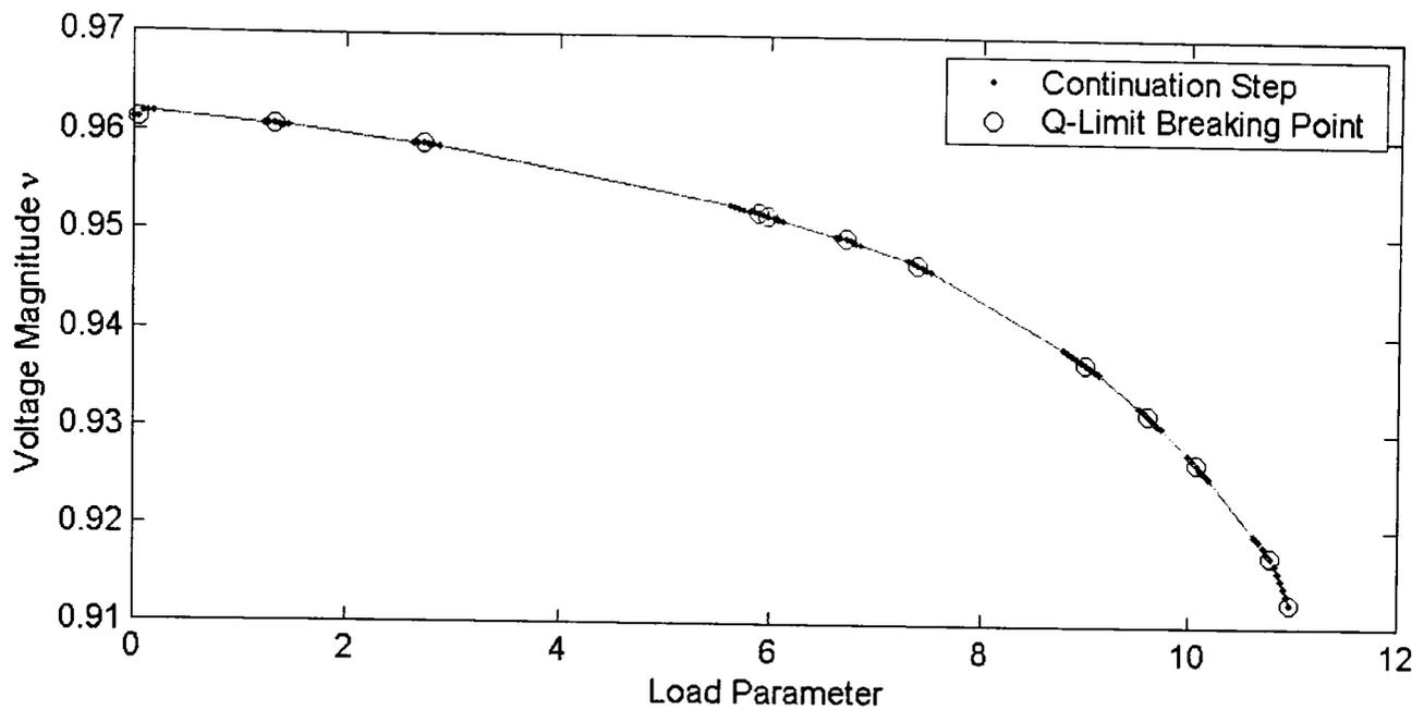
**Figure 6-7-c: Varying single load bus of IEEE 118 bus system using GCPF**
