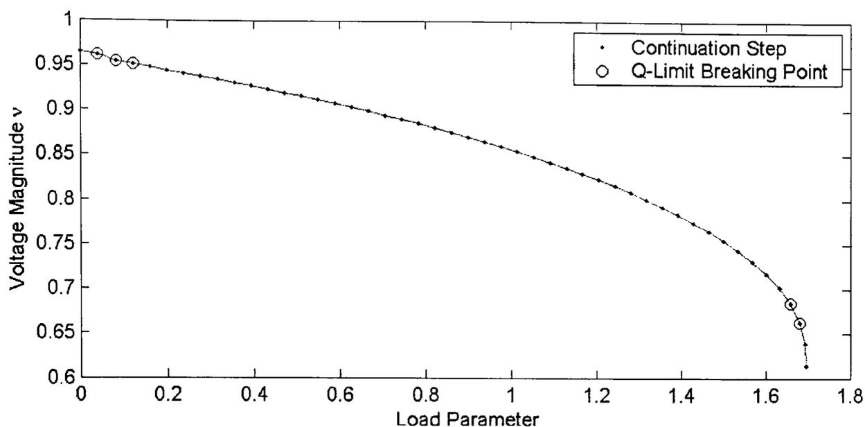
**Figure 6-9-a: Varying single load bus of NGC 61 bus system using CCPF**
