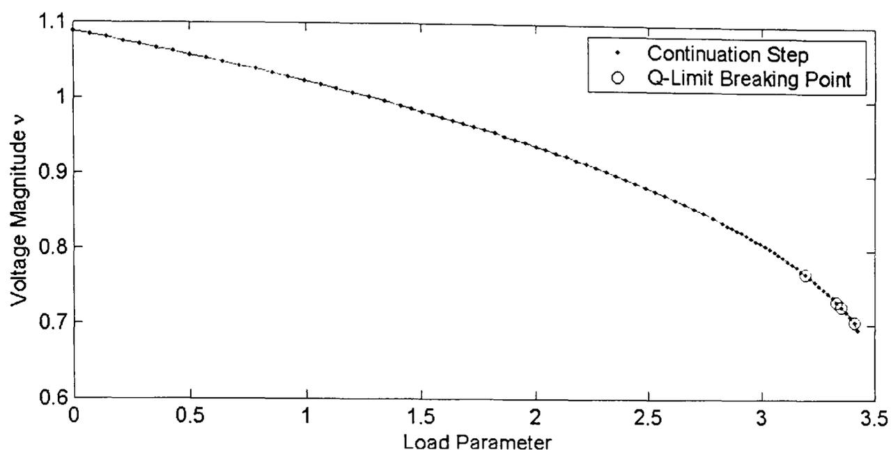
**Figure 6-13-b: Varying multiple load buses in area two of NG 953 using ECPF**
