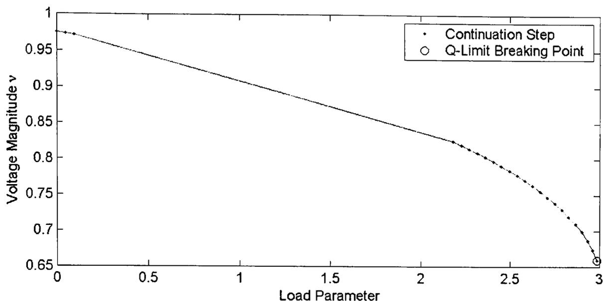
**Figure 6-2-c: Varying single load bus of IEEE 9 bus system using GCPF**
