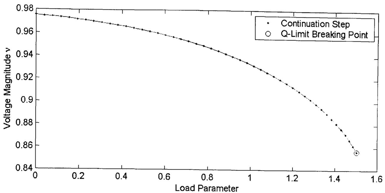
**Figure 6-3-a: Varying multiple load buses of IEEE 9 bus system using CCPF**
