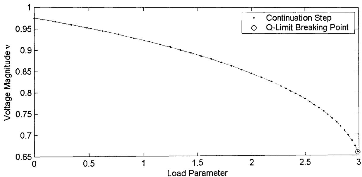
**Figure 6-2-b: Varying single load bus of IEEE 9 bus system using ECPF**
