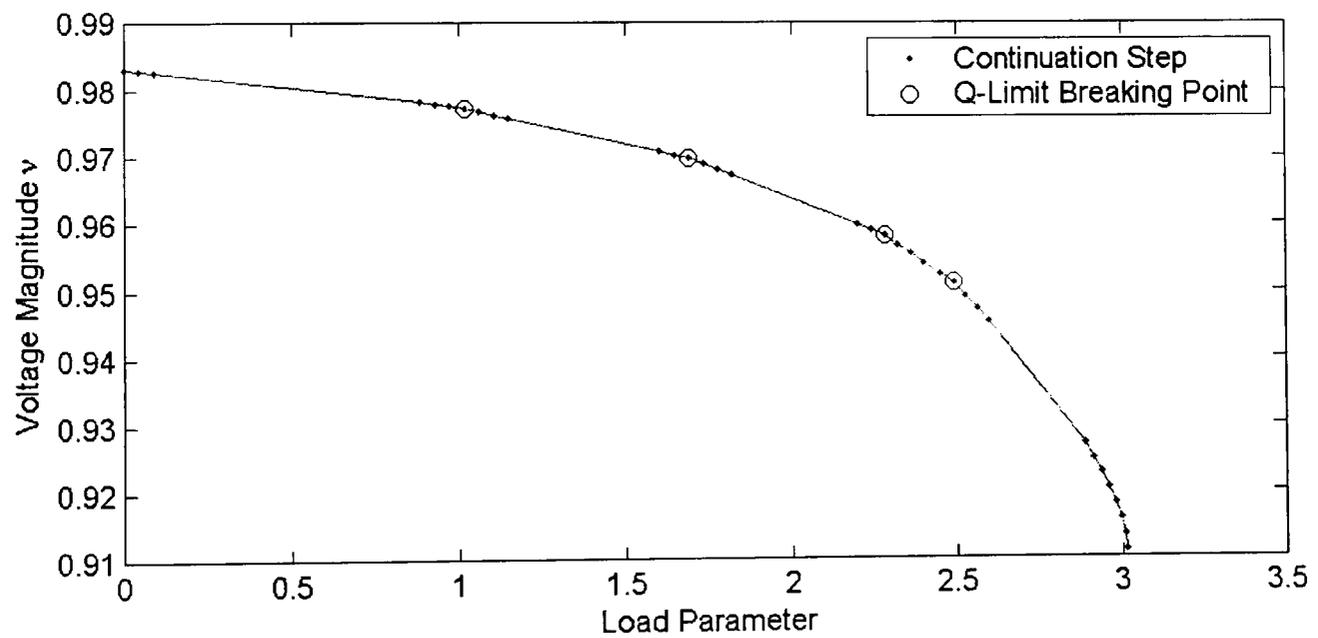
**Figure 6-6-c: Varying multiple load buses of IEEE 30 bus system using GCPF**
