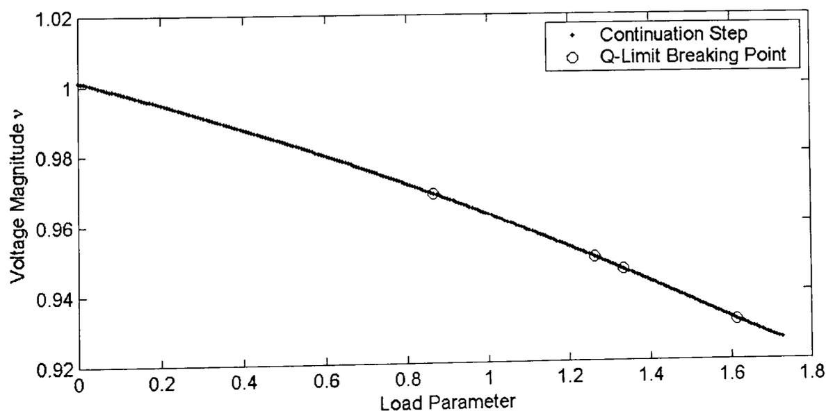
**Figure 6-15: Failure in varying multiple load buses in area four of NG953**
