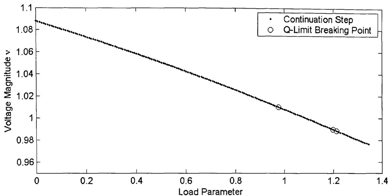
**Figure 6-12: Failure in varying multiple load buses in area two of NG953**
