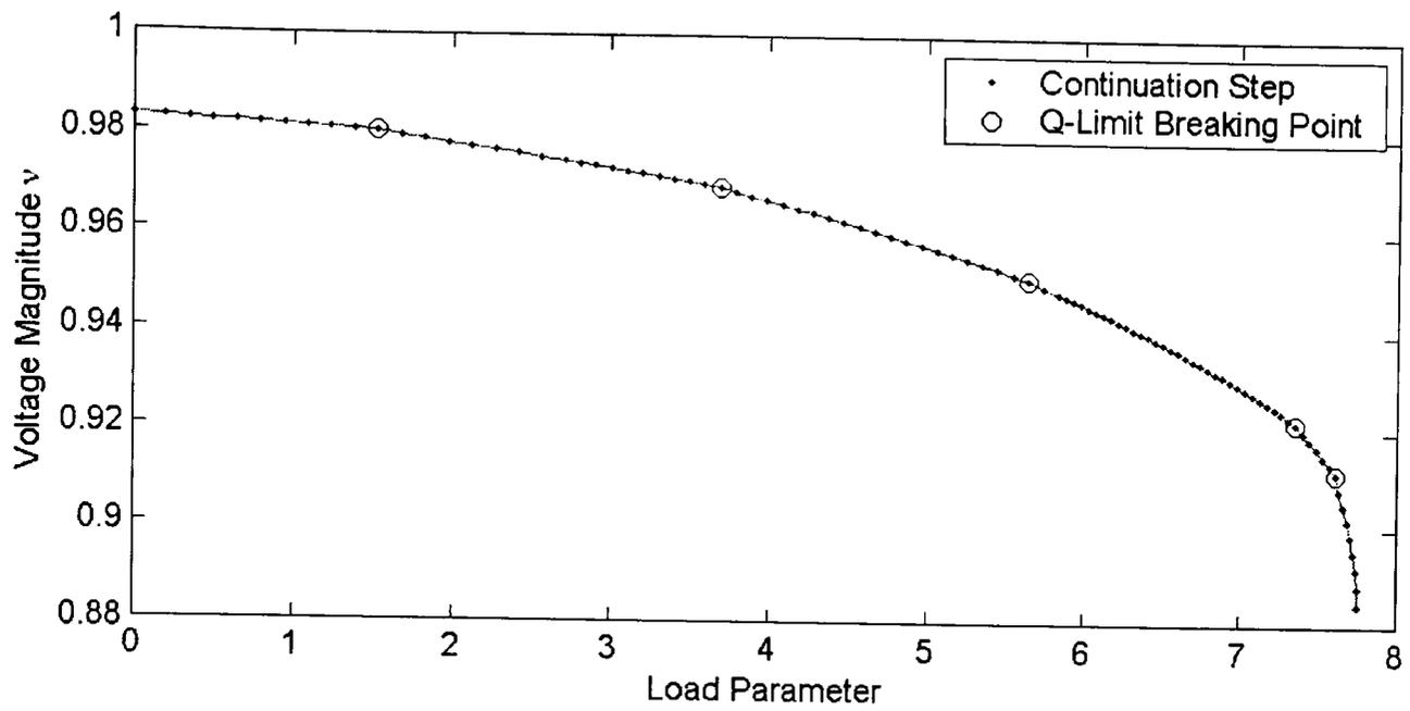
**Figure 6-5-b: Varying single load bus of IEEE 30 bus system using ECPF**
