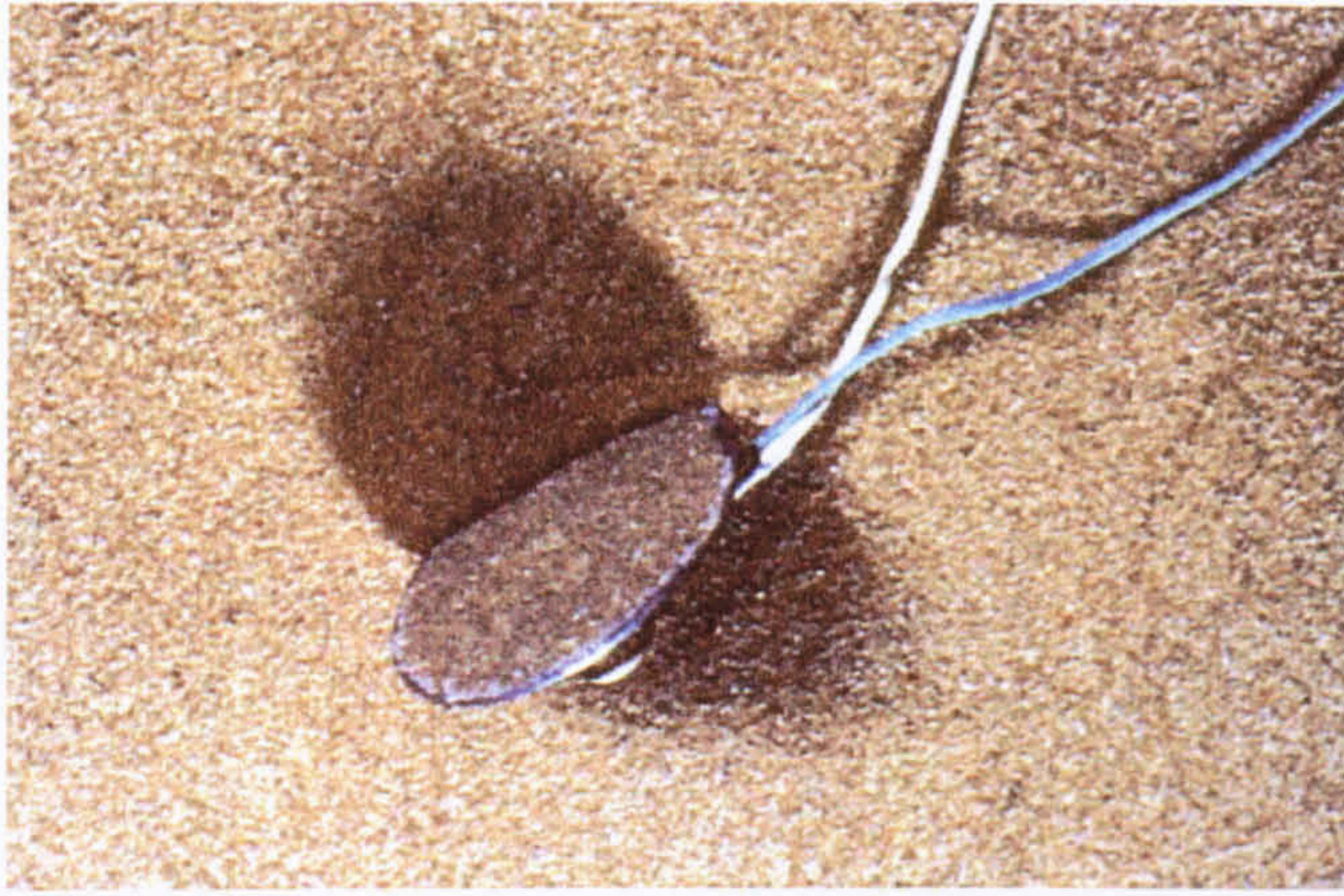
Figure 10.6 – Free field cell of the type designed by Askegaard (1978)
