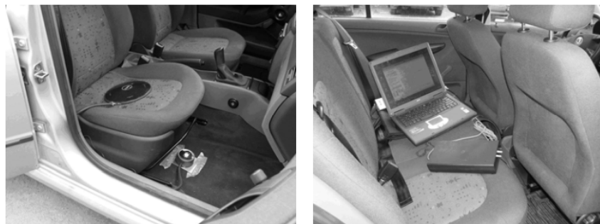
Fig. 109. Set up for the on-road vibration measurement (Stein et al. , 2011)
