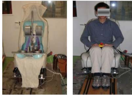
Fig. 103. Laboratory test set up for studying the seat dynamics (Zhang, 2014)
