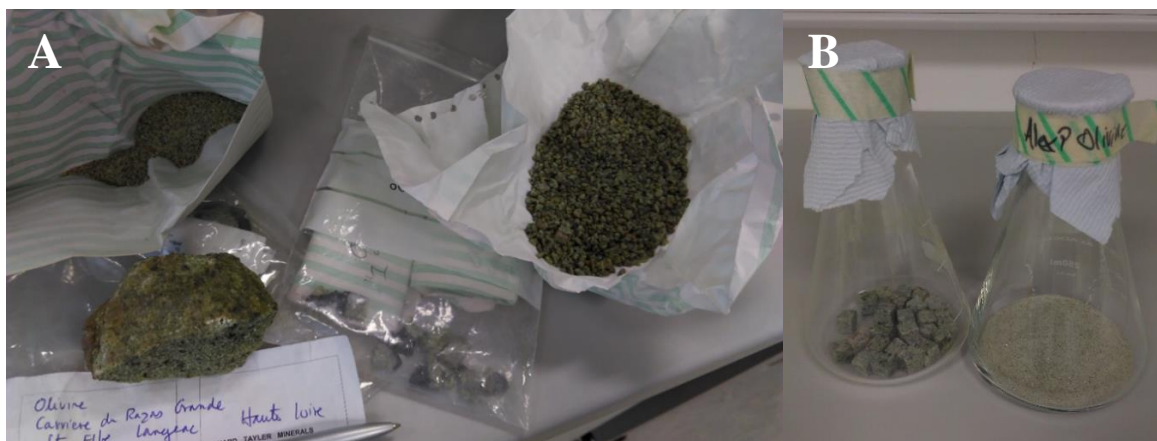
Figure 2.2. Olivine used as the \text{Fe}^{2+} substrate in growth experiments. (A) Fine ( \sim 1 mm) grains (top left), coarse ( \sim 5 mm) granules (right) and main rock sample (bottom left) were processed into (B) a >1 mm powder substrate (right) and 1 \text{ cm}^3 cubes (left).
