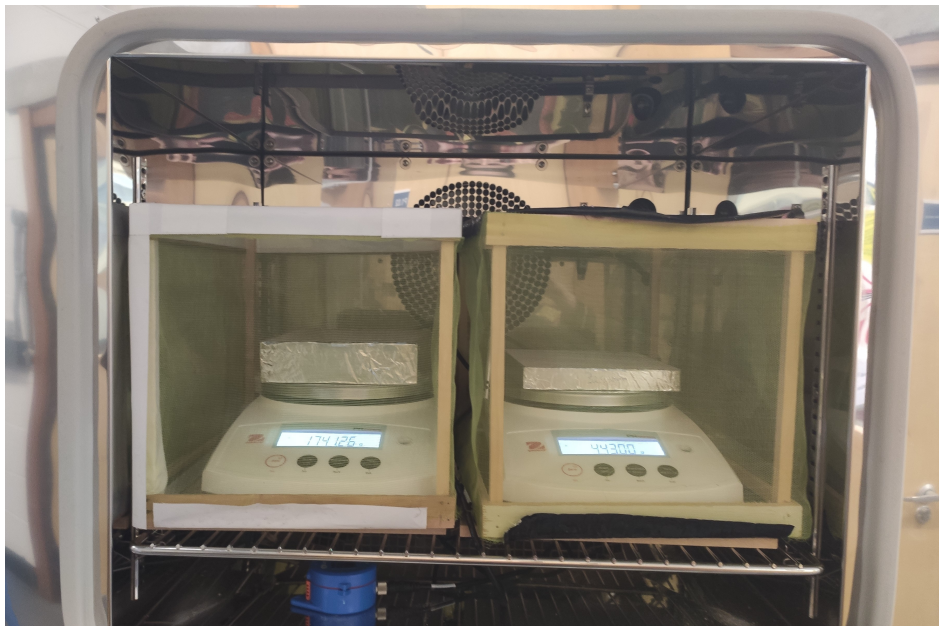
Figure 1. Moisture buffering set up in the climatic chamber
