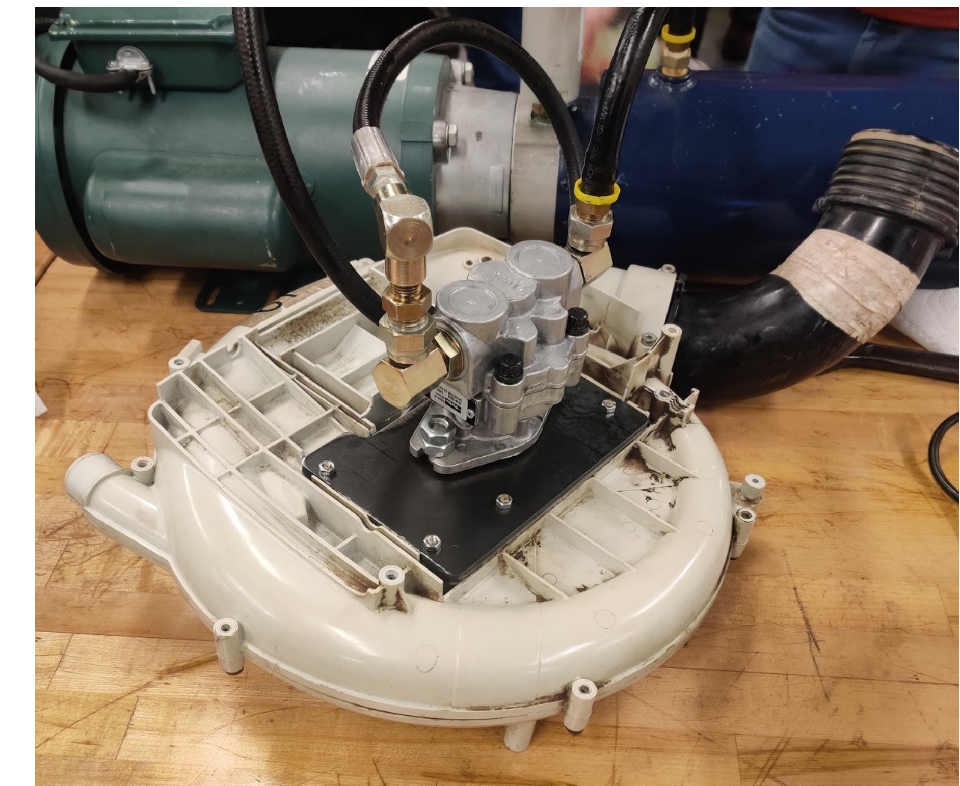
Motor with adapter plate to attached to the Stihl 420 blower
