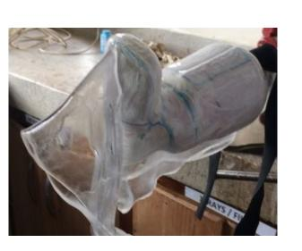
turing method that will hopefully reduce production time and variability at the CURE International Hospital in Kijabe, Kenya where a clinical study is currently being performed. This year, we prototyped a clay mold for wrapping a flat plastic cutout into the shape of the brace. Next year, we plan to improve the process by 3-D printing a
