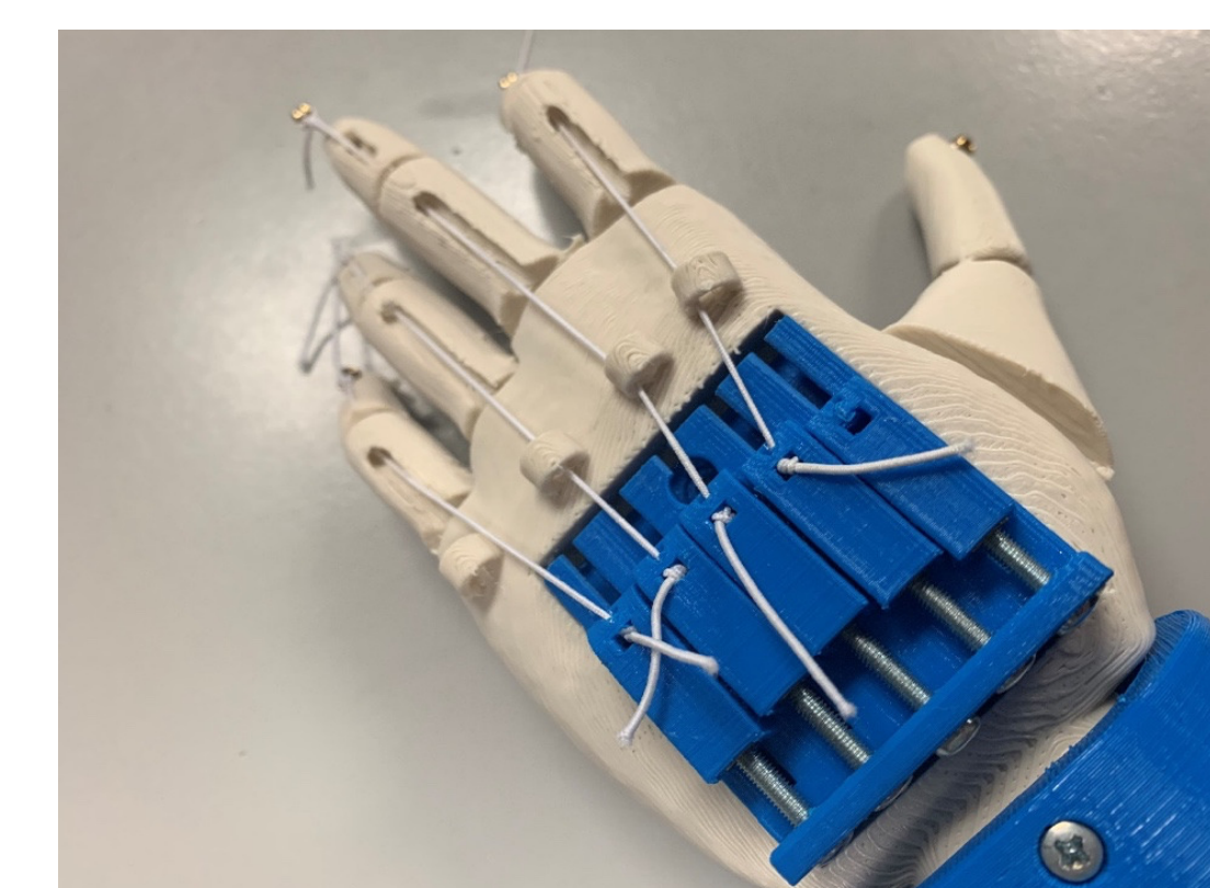
Figure 6: Fully assembled back tension system
