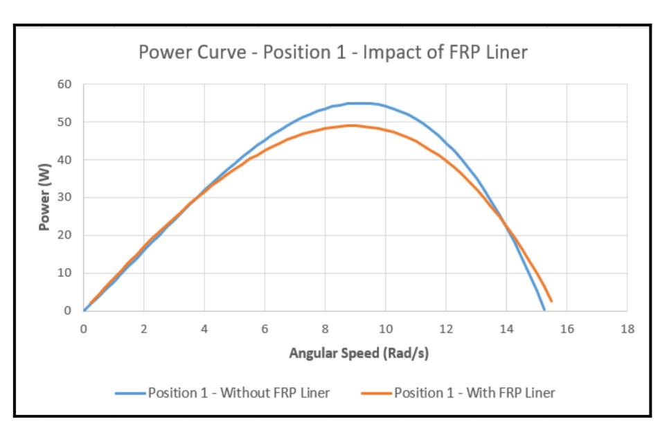
The team thought the addition of a liner would increase power output. However, the power curves to the left show that this was not the case.
