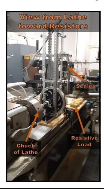
Using the testing set-up to the left, the team determined the efficiency of the chosen generator to be approximately 60.7%
