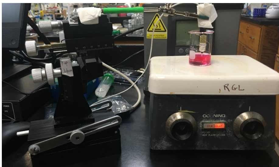
Figure 2-2: Setup of probe during calibration. The magnetic stirrer ensured a continuous flow of \text{H}_2\text{O}_2 to the electrode surface.
