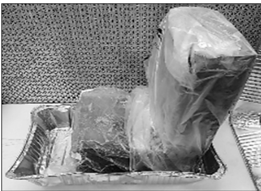
Figure 3. Example of a Douglas-fir connector assembly inoculated with Gloeophyllum trabeum showing minimal fungal growth on the outside of the wood.
