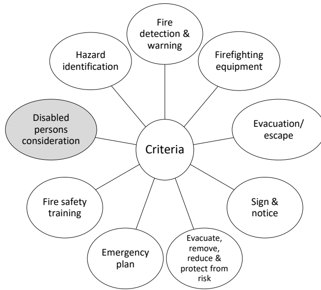
Figure 2: Ten (10) criteria of FRA Adapted from Department for Communities and Local Government (2006)
