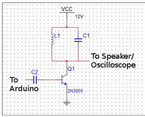
Figure 4. Schematics of the Filter/Amplifier
