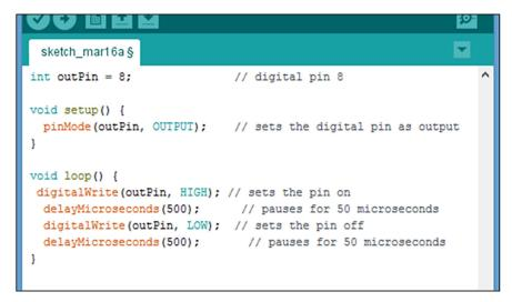
Figure 3. Arduino Program Used to Generate Square Wave
