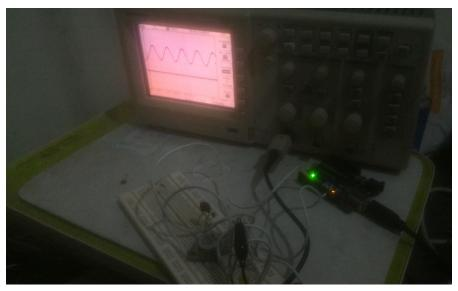
Figure 7. Sine Wave Output from Filter/Amplifier @10KHz
