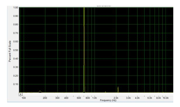
Figure 8. Spectrum Analysis after Filtering @700Hz
