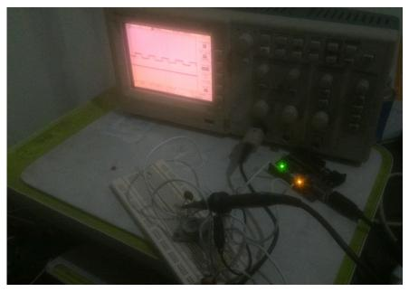
Figure 5. Square Wave Output from Arduino @10KHz
