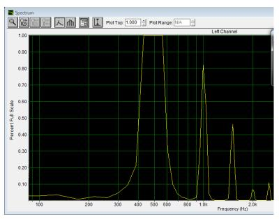
Figure 6. Square Wave Output from Arduino @500Hz
