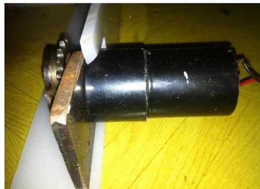
**Gambar 8.** Motor DC 12-24 V
