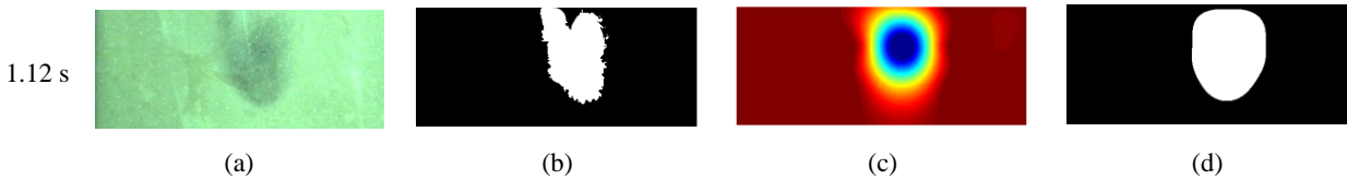
Fig. 8. Images of a bubble at jet gas velocity 6.34 m/s. (a) Original image from the digital camera. (b) Binary image from the digital camera. (c) Image reconstructed from the electrostatic sensor array. (d) Binary image from the electrostatic sensor array.
