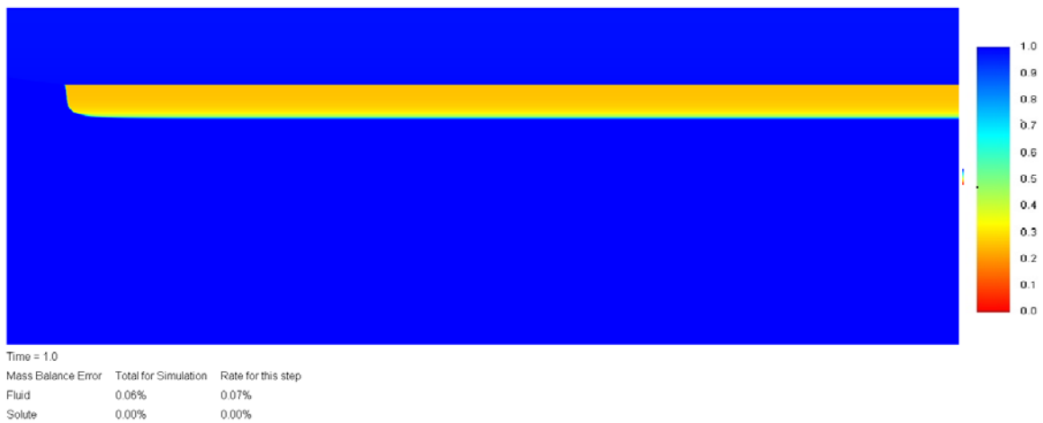
Figure 39: Simulated saturation for low saturated hydraulic conductivity (0.223 m/day) and mid porosity (0.28) for the axisymmetric VS2DTi model
