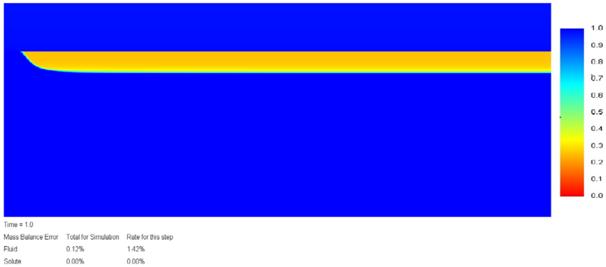
Figure 36: Simulated saturation for mid saturated hydraulic conductivity (2.23 m/day) and mid porosity (0.28) for the axisymmetric VS2DTi model
