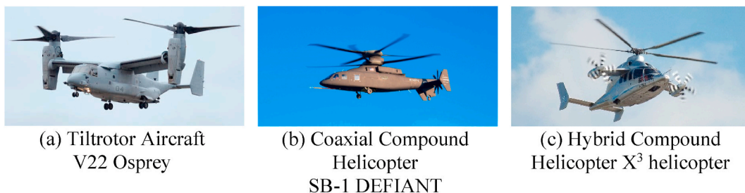
Fig. 1. The primary advanced rotorcraft configurations.
