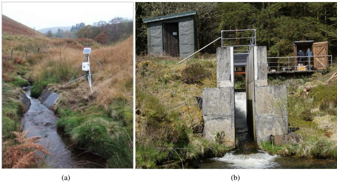
Figure 2.3 (a) FRPB Flume (gauging \sim 1\text{km}^2 at a cost of \sim \pounds 500 ) and (b) CEH mountain flume ( \sim 4\text{km}^2 for \sim \pounds 50,000 ) (These photos are courtesy of a NERC funded presentation by Barry Hankin and Nick Chappell)
