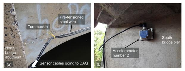
Figure 3.11 (a) cables run on a pre-tensioned wire (b) an accelerometer mounted on the bridge
