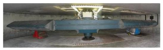
Figure 4.2 Turner beam centrifuge, where all tests were conducted. Photograph from SERIES (2011)
