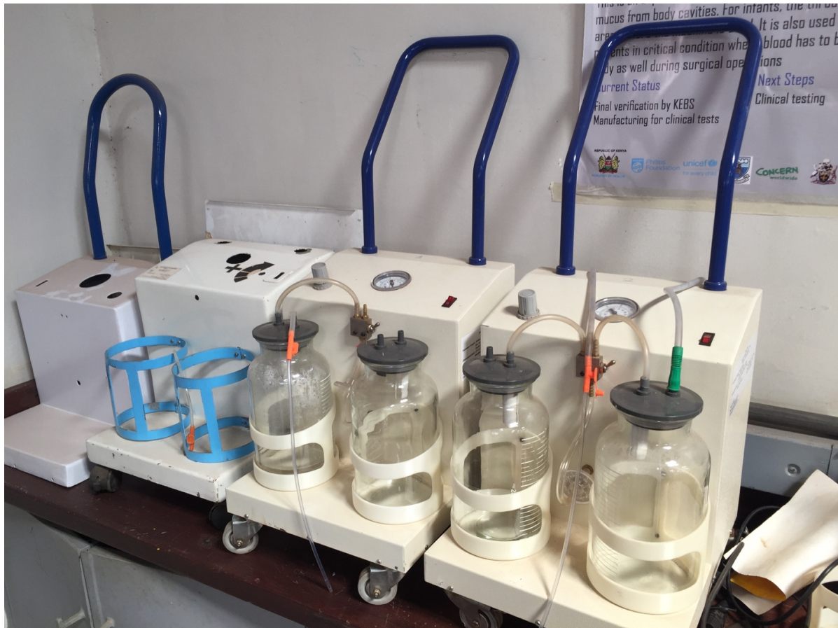
Figure 5.9 – Design evolution of the suction pump machine developed by FabLab/MakerSpace Nairobi
