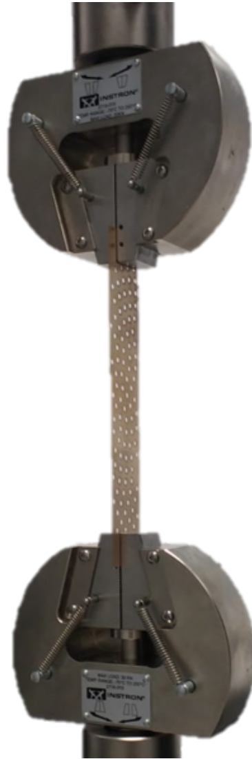
Fig. 4.36 The experimental set-up of the uniaxial tensile loading of a perforated strip. An INSTRON grips the ends of the specimen and imparts a quasi-static displacement, measuring the force response as it does so.
