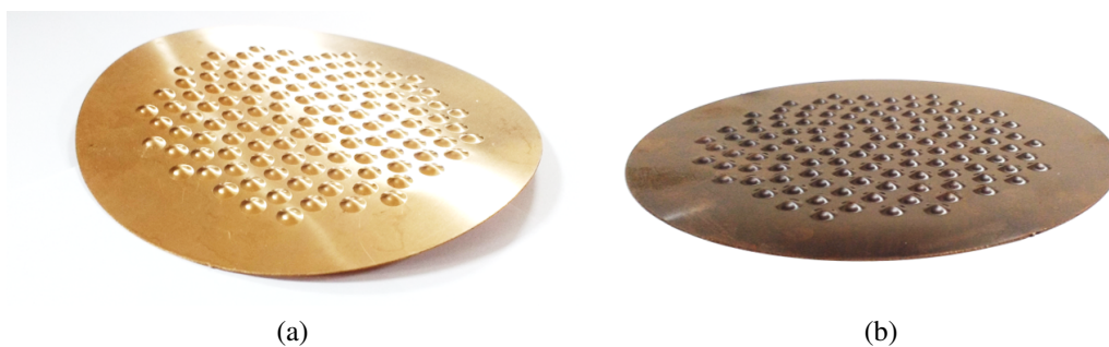
Fig. 5.17 A circular dimpled sheet with a phyllotaxis dimple pattern is shown before and after a heat treatment of 400^\circ\text{C} for 6 hours. (a) Before the heat treatment, the self-stress induce a global curvature. (b) After the heat treatment complete stress relaxation is observed and sheet is globally flat.
