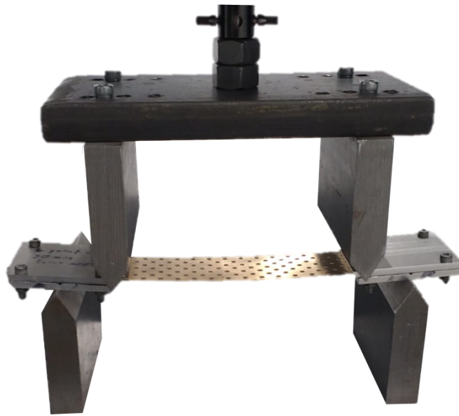
Fig. 4.37 The experimental set-up of the uniaxial bending of a perforated strip. Each edge of the strip is clamped between a pair of aluminium blocks, these blocks are loaded using two pairs of knife-edge supports to develop a central constant moment region.
