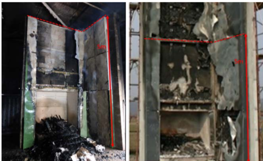
Figure 17 PF/A2 comparison of burn area Čolić (left) and FPA (right) [17]
