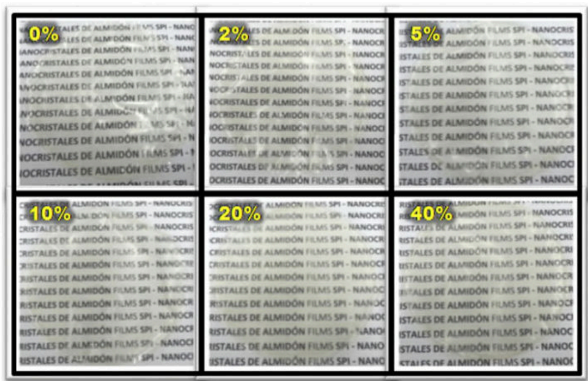
Figure 45. The macroscopic aspect of soy protein isolates films with 0, 2, 5, 10, 20 and 40% w/w of starch nanocrystals. Reproduced with permission from ref 328 . Copyright 2015 Elsevier.
