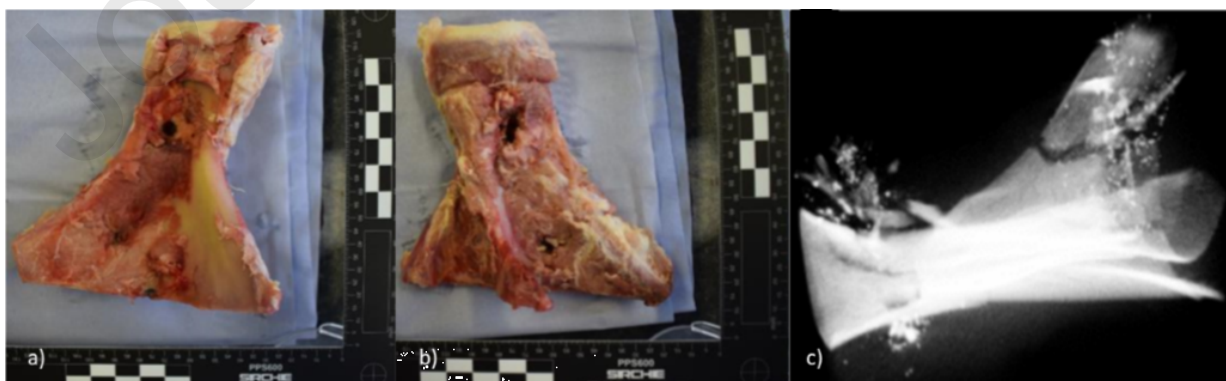
Fig 3: a) Shoulder bone entry wound, b) Shoulder bone exit wound (top flat nose and bottom round nose) and c) Shoulder bone (Micro-CT scan) after being shot (x-ray), round nose (right) and flat nose (left).
