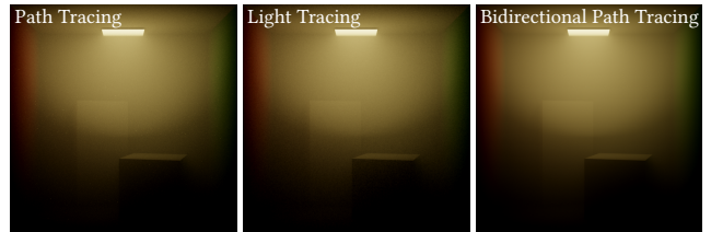
Fig. 11. A homogeneous medium with non-exponential, linearly decreasing transmittance rendered with three different rendering algorithms—path tracing, light tracing and bidirectional path tracing—which were modified to support our theory. All three algorithms produce identical images, which shows that our theory produces consistent results in a bidirectional context, despite being non-reciprocal.
