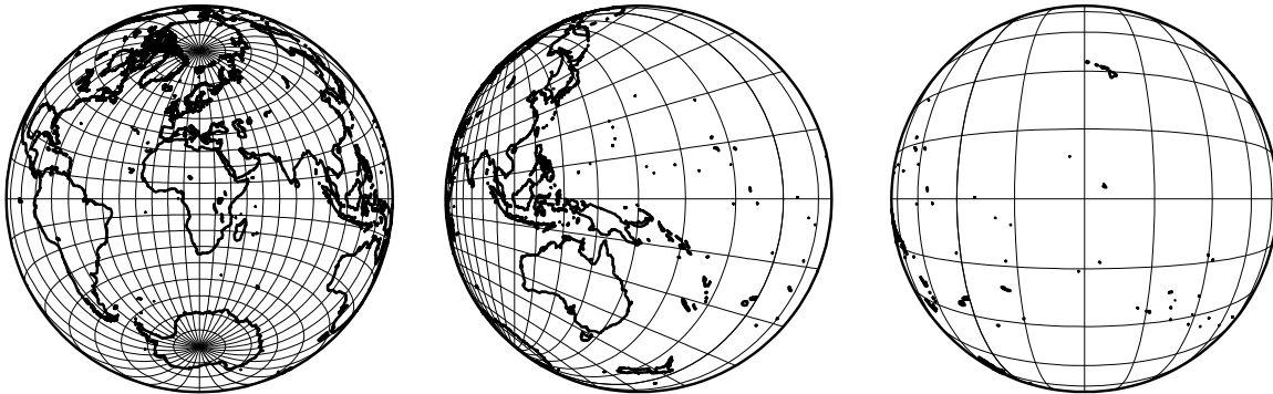
Figure 3. Orthographic views from the front, side, and back of a globe transformed by a droop about (0°N, 20°E). Points on the outer edge of the front view were originally 130° away from the center.
