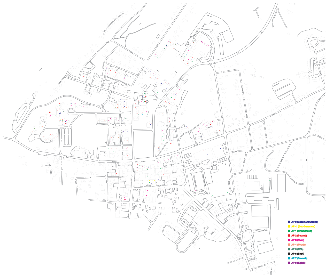
Figure 5: A map of all access points on the Dartmouth College campus. Readers using Acrobat Reader can zoom and pan to see full detail. Note, however, that this two-dimensional map does not clearly show all APs, because some multi-story buildings place APs at the same location on multiple floors.
